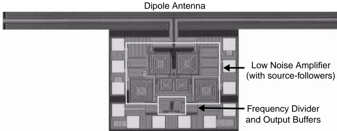
Figure 6-8 Die photograph of 0.25- $\mu\text{m}$  clock receiver with linear dipole antenna.
