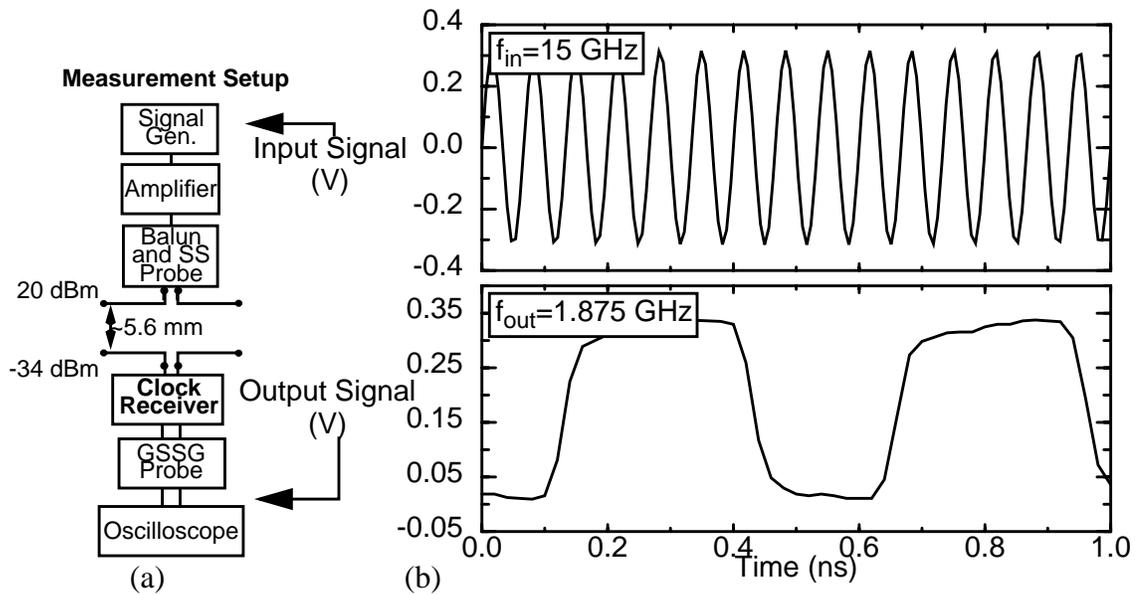
Figure 6-26 (a) Measurement setup used to characterize wireless clock receiver.
