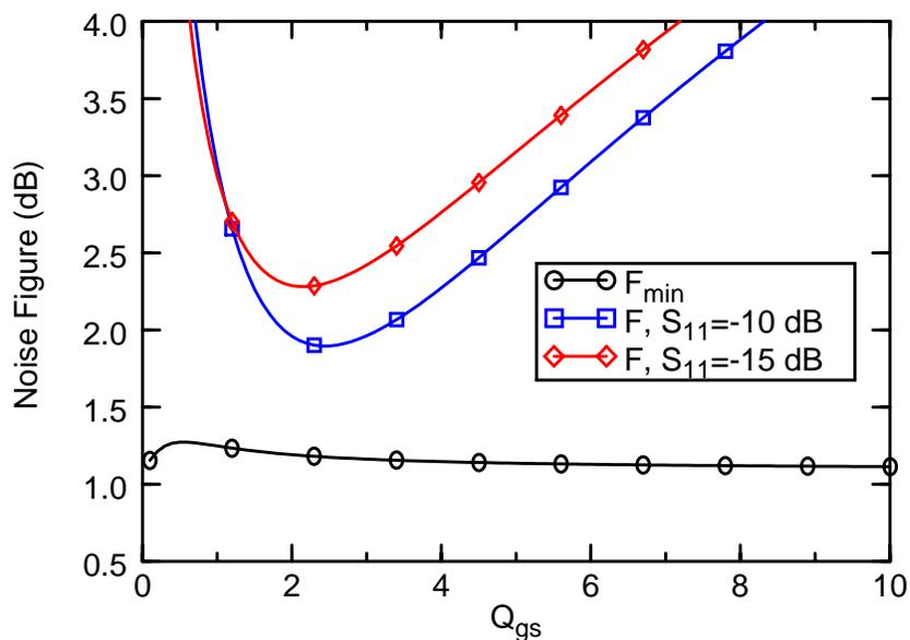
Figure 2-8 Minimum noise figure and actual noise figure when the input matching is constrained by  $S_{11}$ . The difference between  $F$  and  $F_{\min}$  indicates that constraining  $S_{11}$  causes a noise mismatch.
