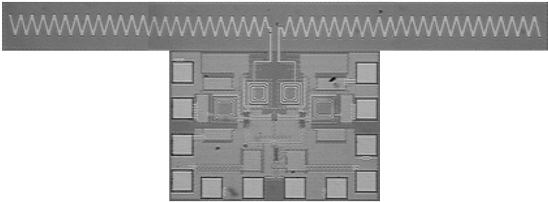
Figure 6-25 Die photograph of 0.18- $\mu\text{m}$  clock receiver with zigzag dipole antenna.
