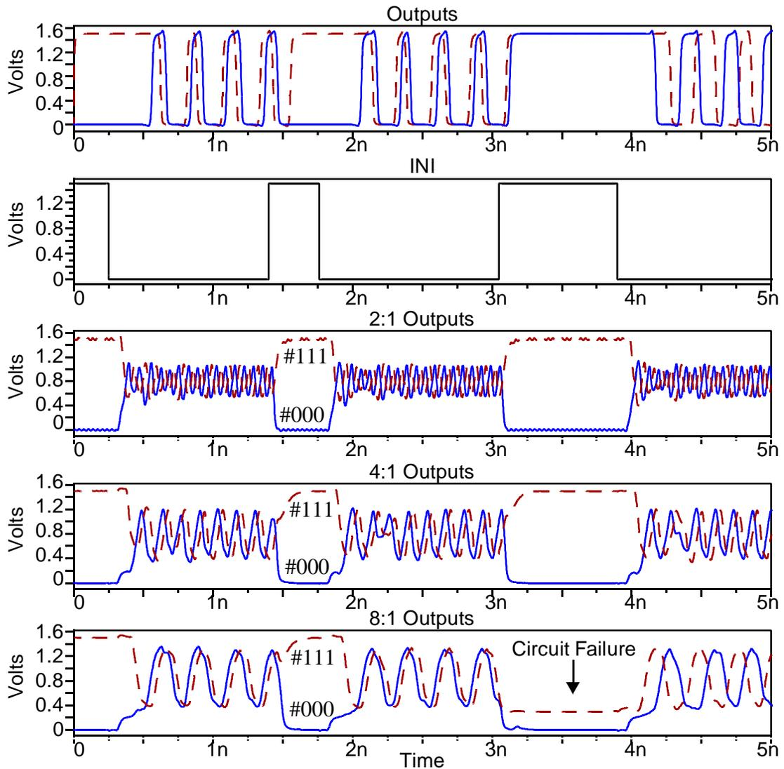
Figure 4-22 Simulated waveforms of two programmable 8:1 dividers--programmed to #000 (solid lines) and #111 (dashed lines)--for repeated initializations. On the third initialization the circuit fails, as indicated.
