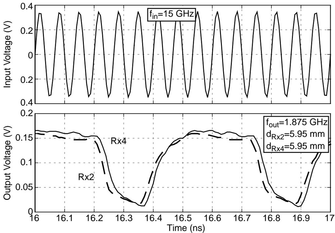
Figure 6-28 Measured input and output waveforms of double-receiver interconnect using  $Z_{6b}$  as the transmitting antenna, with a wood as the back dielectric. Input frequency is 15 GHz; output frequencies are 1.875 GHz; distances are 5.95 mm, each.
