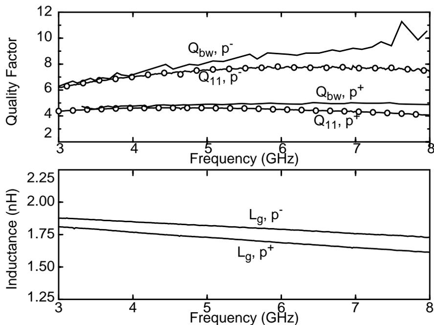
Figure 3-9 Quality factors and inductance of  $L_g$  versus frequency for different substrate resistivities ( $p^+ \sim 0.01 \Omega\text{-cm}$ ,  $p^-$  with epi  $\sim 8 \Omega\text{-cm}$ ). The inductor is implemented in a 5-metal-layer 0.25- $\mu\text{m}$  CMOS process.
