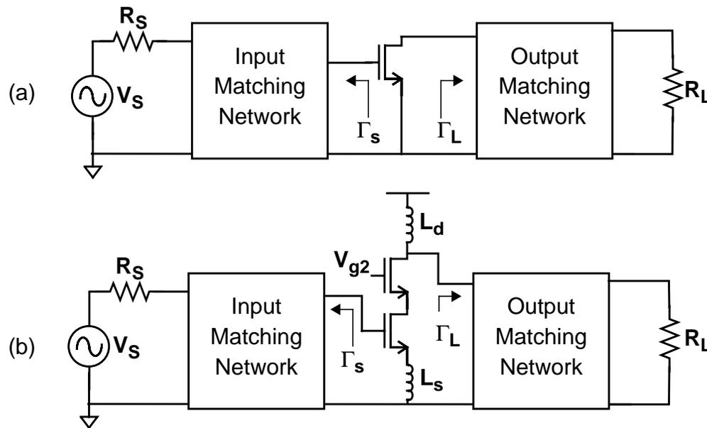
Figure 2-10 Illustration of constant available gain methods, where for the gain stage either, (a) a single transistor is used or (b) a source-degenerated cascode with inductive load is used.
