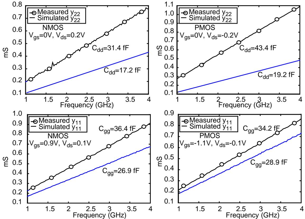
Figure 3-15 Measured versus simulated  $y_{11}$  (with transistor in linear region) and  $y_{22}$  (with transistor off) for NMOS and PMOS transistors. The slope of these lines over  $2\pi$  is equal to the capacitances  $C_{gg}$  and  $C_{dd}$  for  $y_{11}$  and  $y_{22}$ , respectively.
