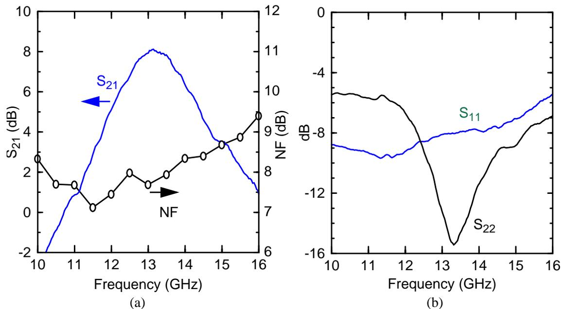
Figure 3-16 (a) Measured gain and noise figure for 0.18- $\mu\text{m}$  LNA.
