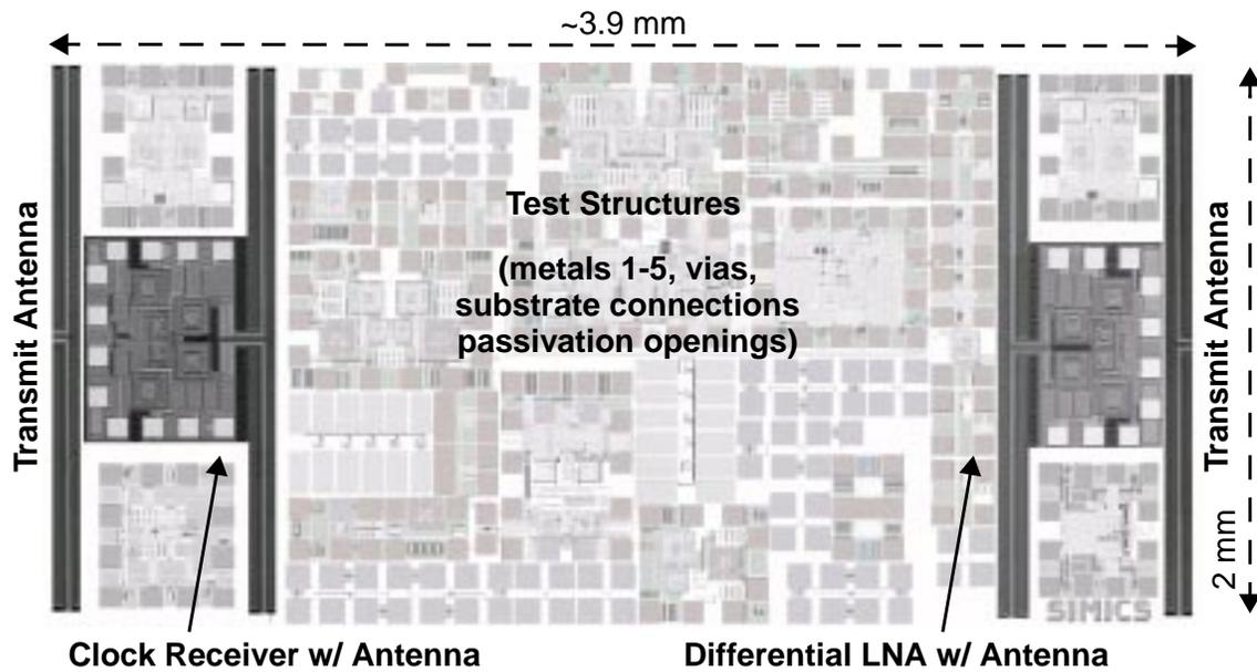
Figure 6-3 Photo-illustration of 0.25- $\mu\text{m}$  test-chip including antenna pair, antenna with LNA, and antenna with clock receiver.
