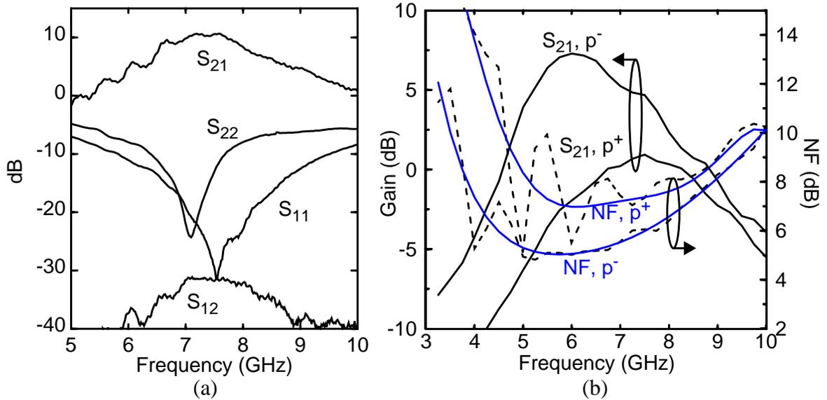
Figure 3-10 (a) Measured S-parameters of differential LNA. (b) Measured gain and NF for single-ended NF for both p<sup>+</sup> and p<sup>-</sup> substrates.
