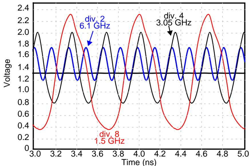
Figure 4-3 Simulation of self-oscillation of 8:1 source-coupled divider. The clock inputs are held at 1.3 V, causing the first 2:1 divider to oscillate at 6.1 GHz for  $V_{dd}=2.5$ V ( $f_{iSO} = 12.2$  GHz).
