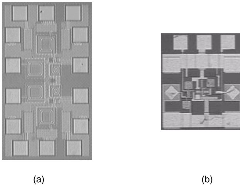
Figure 3-13 Die photographs of (a) 0.18- $\mu\text{m}$ , 14-GHz differential CMOS LNA and (b) 0.1- $\mu\text{m}$ , 23.8-GHz SOI CMOS tuned amplifier.
