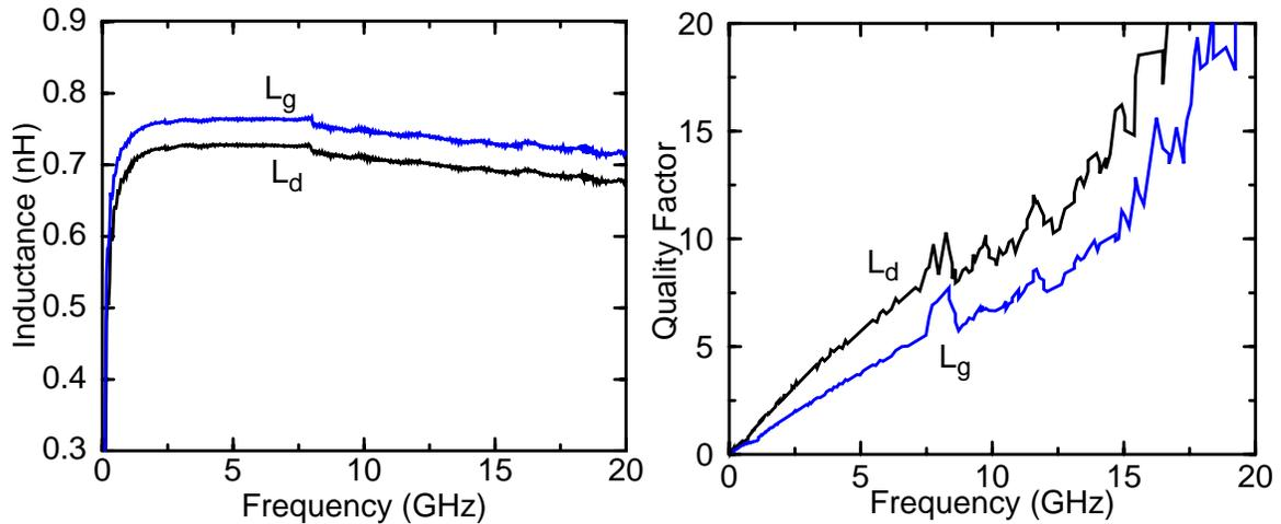
Figure 3-14 Measured (a) inductance and (b) quality factor ( $Q_{bw}$ ) for  $L_g$ , and  $L_d$ .
