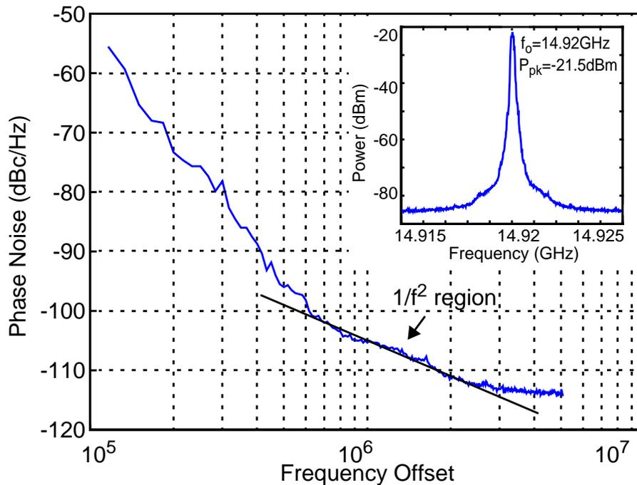
Figure 6-20 Single-sideband plot for 0.18- $\mu\text{m}$  VCO with output spectrum inset.
