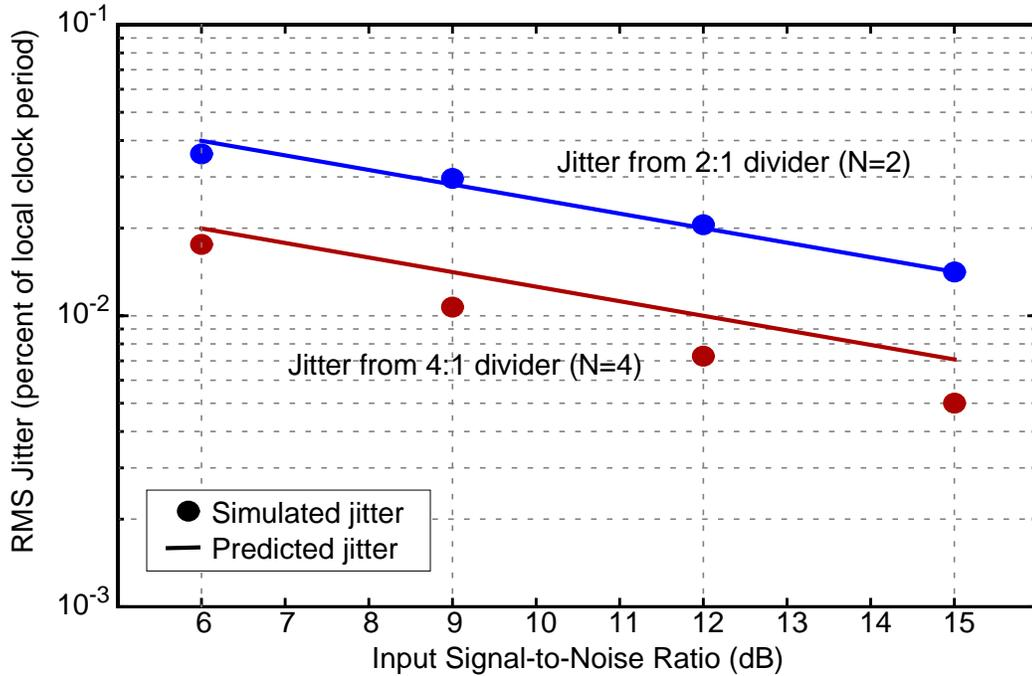
Figure 5-8 Simulation results of RMS jitter versus input SNR from 0.25- $\mu\text{m}$  frequency divider after a division by 2 and division by 4. The simulated jitter (points) is compared to the predicted jitter (line) from (5.35).
