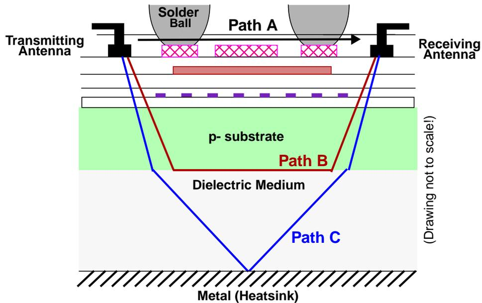
Figure 6-2 Cross-sectional illustration of chip for metal antennas with interference structures. Three possible signal paths between antennas--path A is direct path, path B is substrate surface wave, and path C is substrate reflection.
