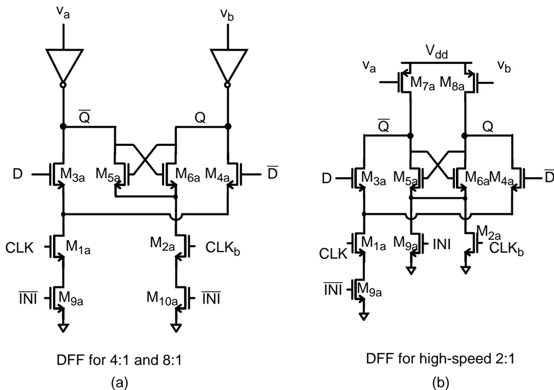
Figure 4-24 (a) Schematic of fixed programmable DFF (for lower frequency divide-by-4 and divide-by-8). (b) Schematic of improved high-frequency (divide-by-2) programmable DFF.
