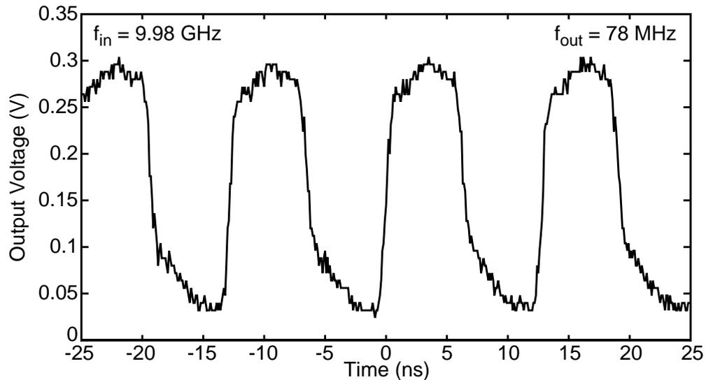
Figure 4-10 Measured output waveform from 0.25- $\mu\text{m}$  CMOS 128:1 frequency divider. Input frequency is 9.98 GHz for  $V_{\text{dd}} = 2.5$  V and output frequency is 78 MHz.
