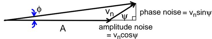
Figure 5-6 Phasor diagram for additive noise, showing how phase noise is generated.
