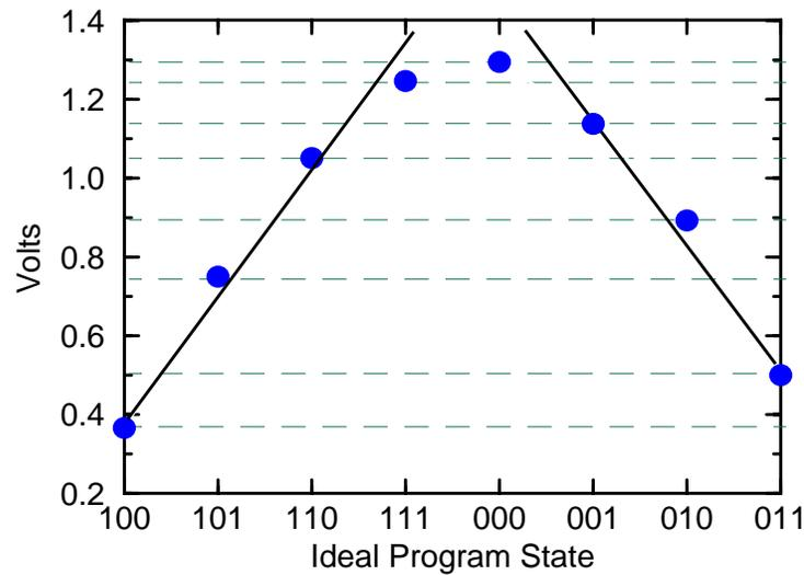
Figure 4-27 Measured outputs of phase detector used to characterize initialization circuitry.
