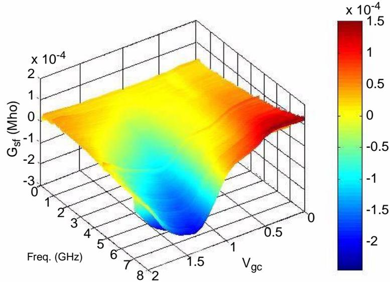
Figure 3-19 Input conductance to source-follower buffer driving a capacitive load versus frequency and control voltage.
