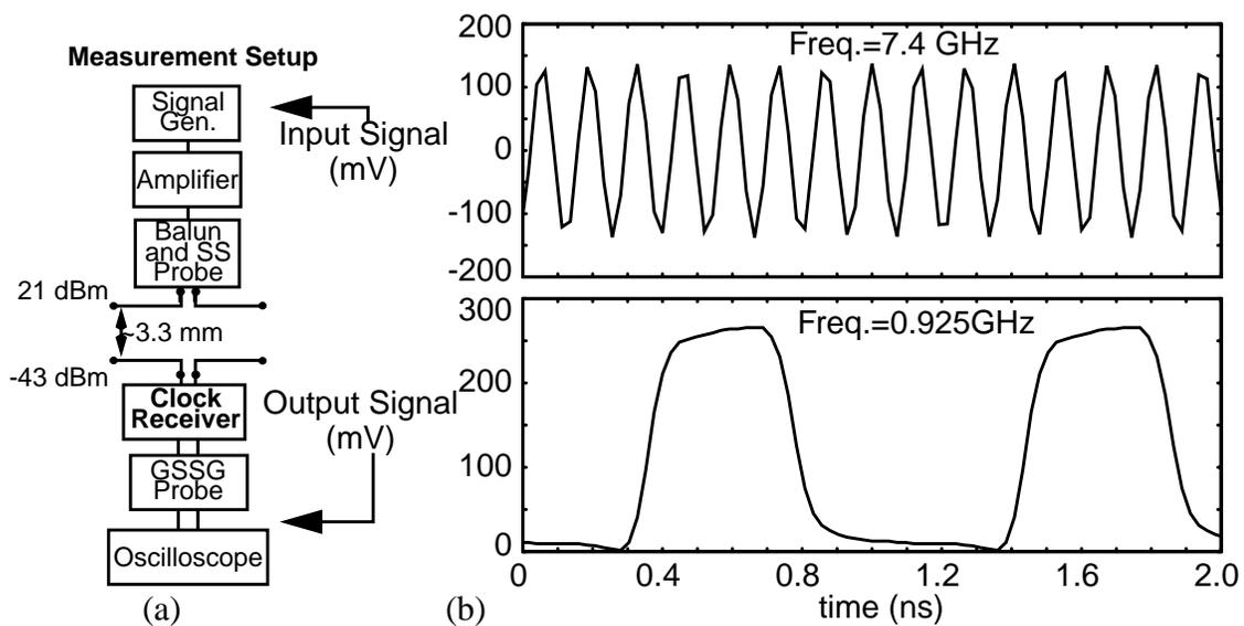
Figure 6-9 (a) Measurement setup used to characterize clock receiver. (b) Input and output waveforms for the clock receiver ( $f_{in}=7.4$  GHz and  $f_{out}=7.4$  GHz/8 = 925 MHz) for a interconnection distance of 3.3 mm.
