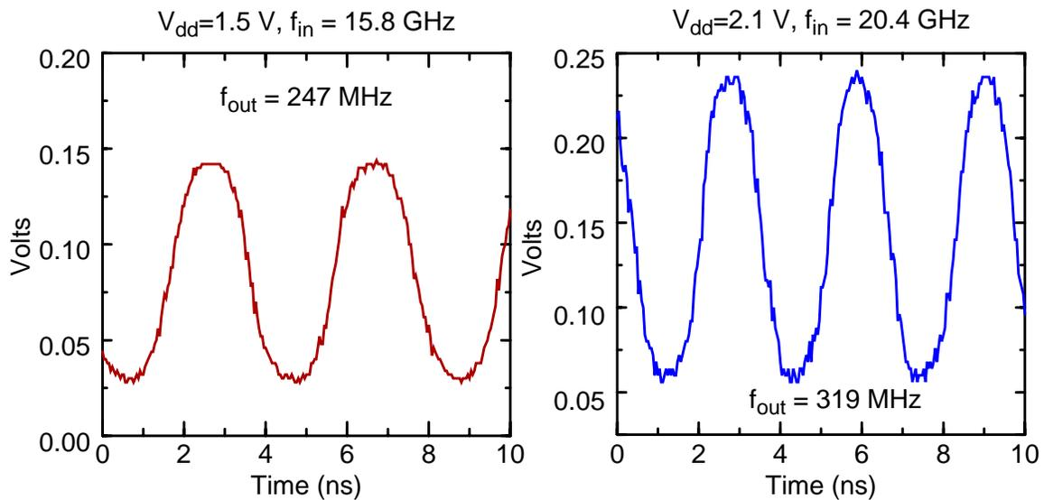
Figure 4-14 Measured output waveforms of 0.18- $\mu\text{m}$  64:1 frequency divider.
