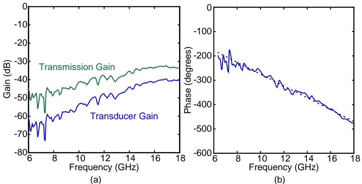
Figure 6-5 (a) Transducer and transmission gain of linear dipole antenna pair. (b) Phase versus frequency for linear dipole antenna pair.
