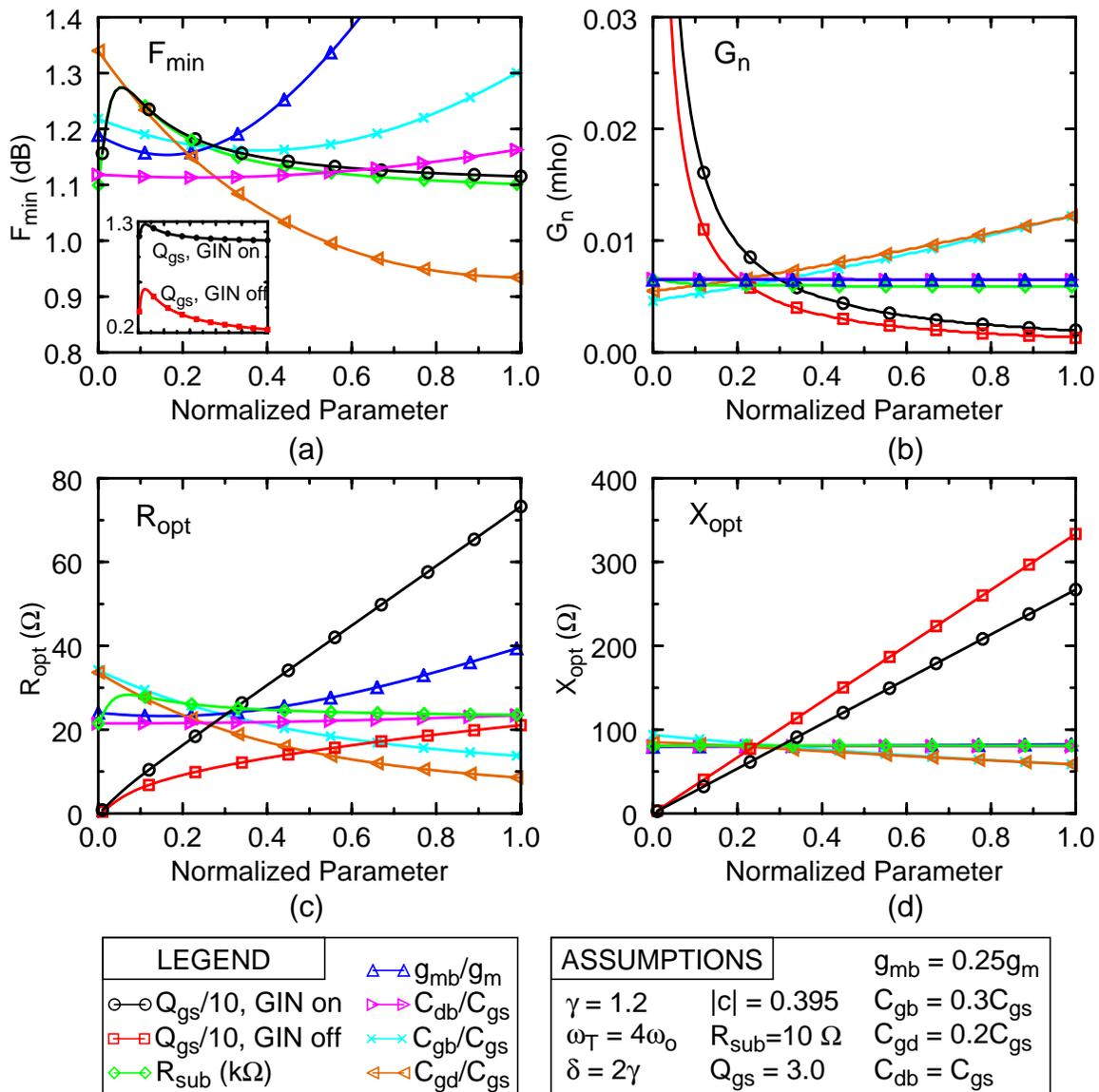
Figure 2-7 Noise parameters (a)  $F_{min}$ , (b)  $G_n$ , (c)  $R_{opt}$ , and (d)  $X_{opt}$ , for the following normalized parameters:  $Q_{gs}$  with GIN on and off,  $R_{sub}$ ,  $g_{mb}$ ,  $C_{db}$ ,  $C_{gb}$ , and  $C_{gd}$ . For each parameter studied, all other parameters are held constant using the values listed in the assumption table, and GIN is on (except, obviously, for  $Q_{gs}$ , GIN off case).
