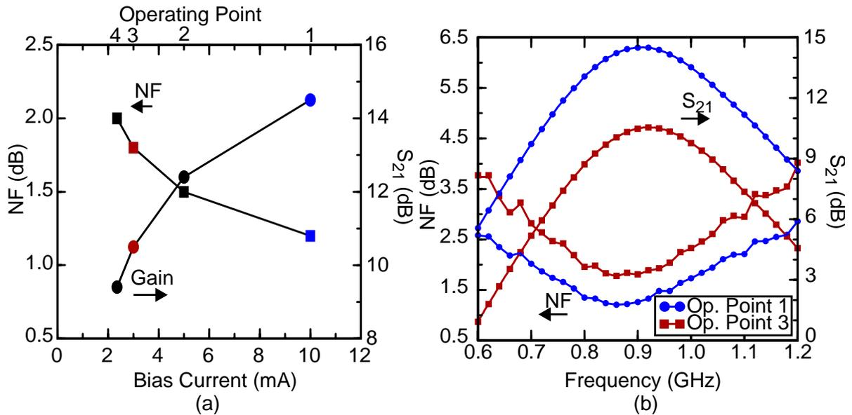
Figure 3-4 (a) Measured gain ( $S_{21}$ ) and noise figure (NF) versus bias current. Four different operating points are shown, numbered 1 to 4, corresponding to minimum to maximum NF and maximum to minimum current, respectively. (b) Gain and NF versus frequency for operating points 1 & 3.
