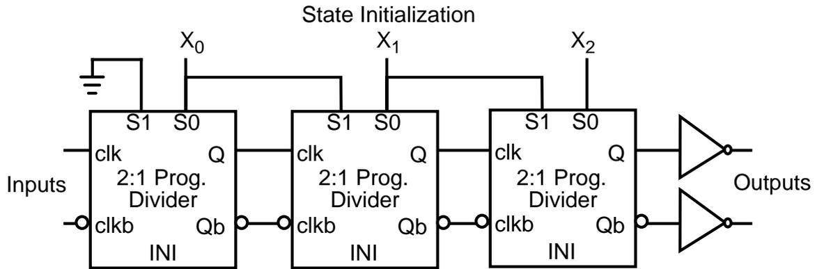
Figure 4-20 Block diagram of programmable 8:1 frequency divider
