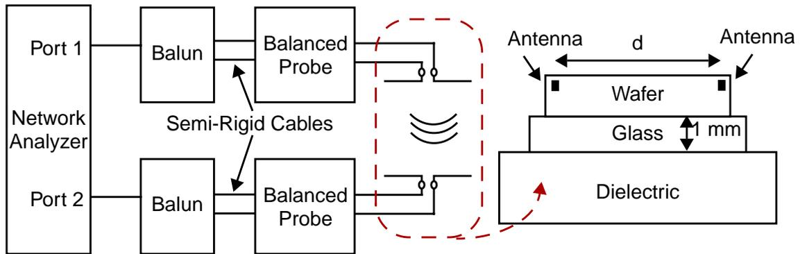
Figure 6-4 Measurement setup used to characterize on-chip antenna pair. On-wafer measurements are performed with the die mounted on a glass slide above a dielectric insulator.
