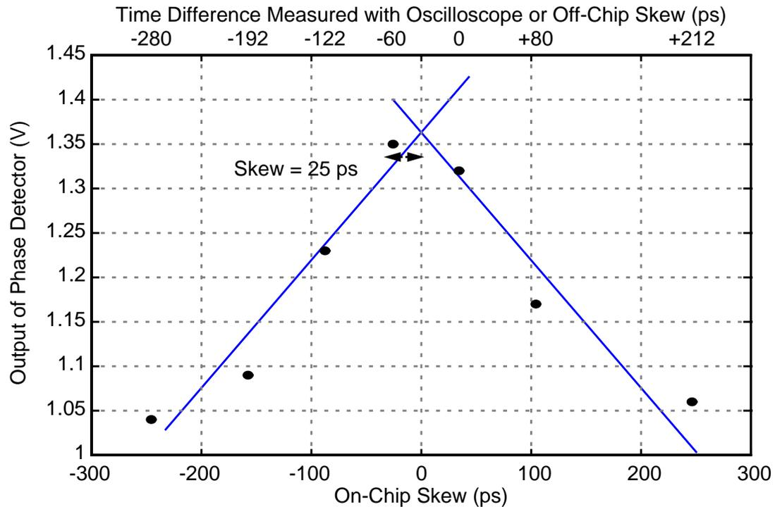
Figure 6-30 Measured output of phase detector versus time difference (skew) measured between waveforms from Rx2 and Rx4 using oscilloscope. Lines with equal and opposite slopes are fit to both the positive and negative portions of the curve, where the lines intersect at the point of zero skew.
