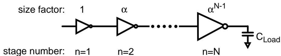
Figure 7-2 Schematic of tapered buffer used in global clock distribution. Each stage is  $\alpha$  times as large as the previous buffer stage, resulting in minimum delay.
