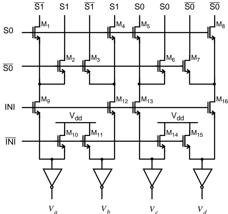
Figure 4-19 Schematic of initialization circuitry implemented with complementary pass-transistor logic.
