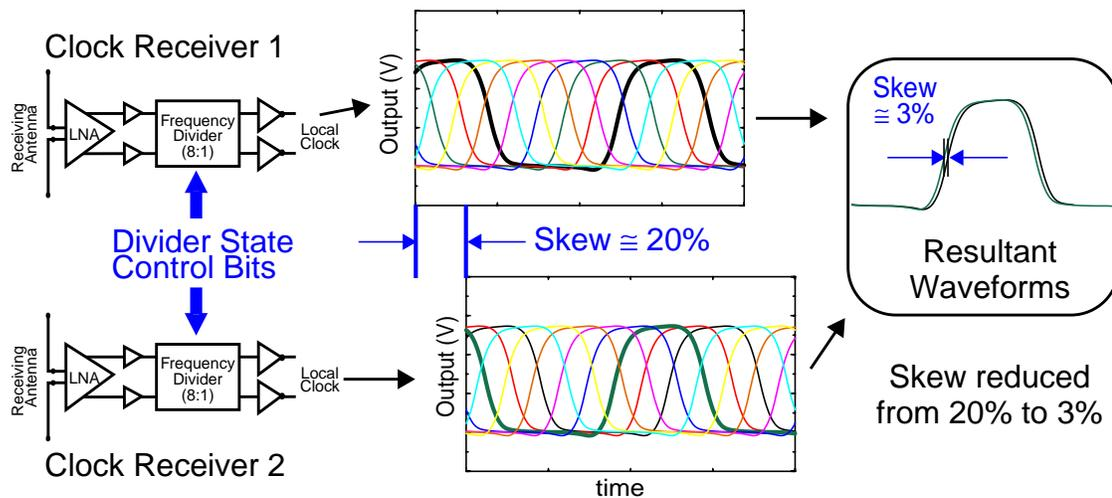
Figure 4-16 Illustrations of concept of divider programming to reduce systematic skew. Two receiver start with a skew of 20% and by selecting the correct state of each, the skew can be reduced to 3% (for this example).
