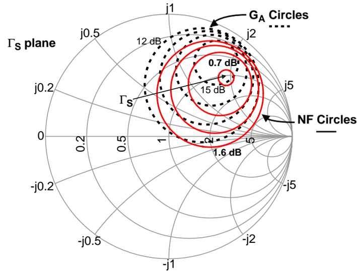
Figure 2-11 Constant available gain and NF circles for cascode with  $L_s$  and  $L_d$ .
