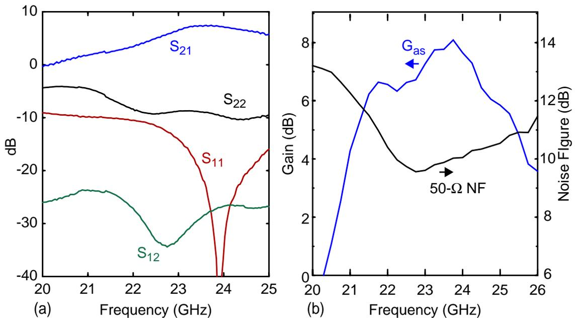
Figure 3-20 (a) Measured S-parameters and (b) measured operating power gain ( $G_p$ ) and 50- $\Omega$  noise figure (NF) vs. frequency.
