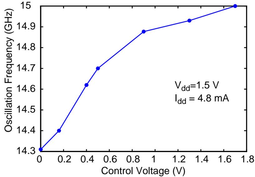
Figure 6-21 Measured tuning range for 0.18- $\mu\text{m}$  VCO.
