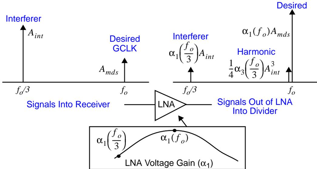
Figure 5-10 Illustration of scenario used to specify LNA IIP3.
