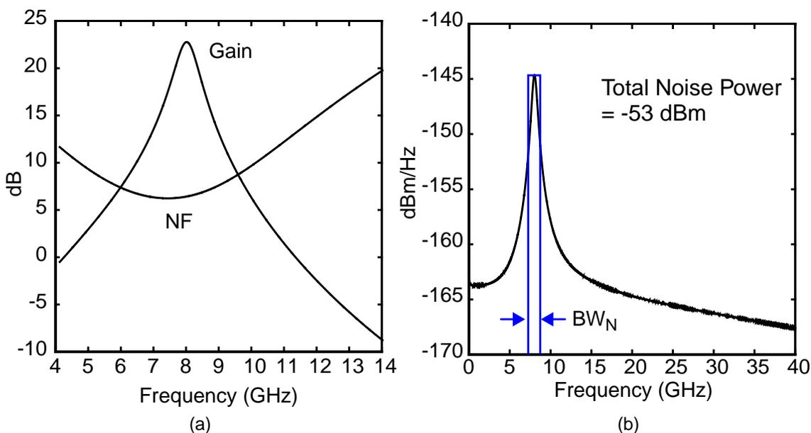
Figure 5-9 (a) Simulated gain and noise figure for 0.25- $\mu\text{m}$  LNA with source-followers. (b) Simulated power spectral density of thermal noise at input of frequency divider, along with equivalent noise bandwidth ( $BW_N$ ).
