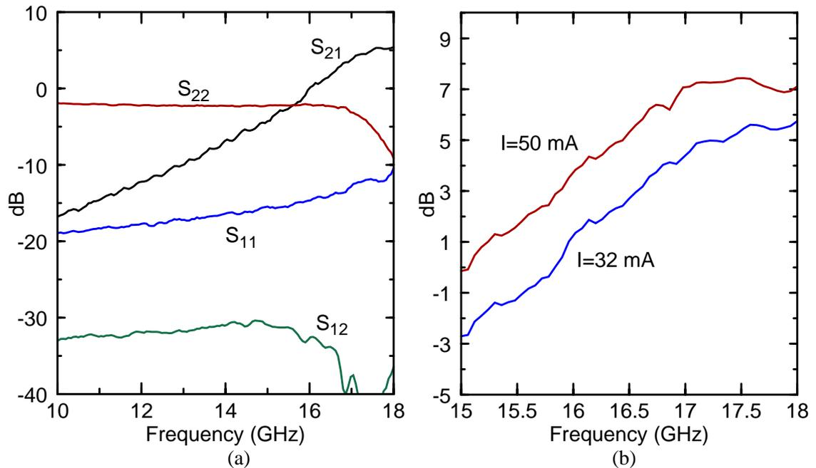
Figure 6-23 (a) S-parameters of power amplifier (driving 50- $\Omega$  differentially).
