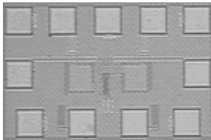
Figure 4-12 Die photograph of 0.18- $\mu\text{m}$ , 64:1, 15.8-GHz source-coupled divider.
