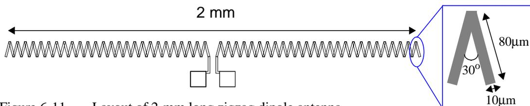
Figure 6-11 Layout of 2-mm long zigzag dipole antenna
