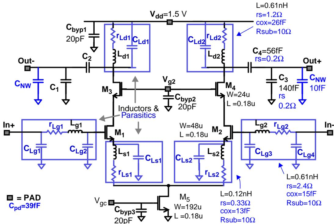
Figure 3-11 Schematic of 14-GHz fully differential LNA showing parasitics.
