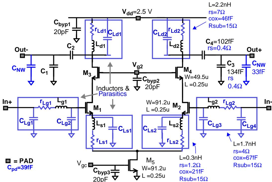
Figure 3-8 Schematic of 8-GHz fully differential LNA showing parasitics.
