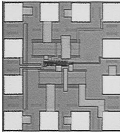
Figure 4-7 Die photograph of 0.25- $\mu\text{m}$ , 128:1, 10-GHz source-coupled divider.
