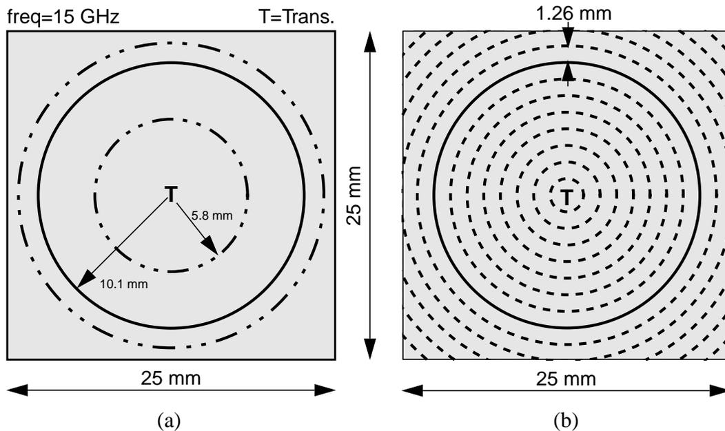
Figure 4-15 Illustrations (to scale) of grids upon which clock receivers should be placed. (a) Grid spacing of one wavelength from transmitter, with solid for wavelength in silicon dioxide and dash-dot for wavelength in silicon. (b) Grid spacing of one eighth of a wavelength in oxide, used when the dividers are programmed to initial states of 0 to 7 (for divide-by-8).
