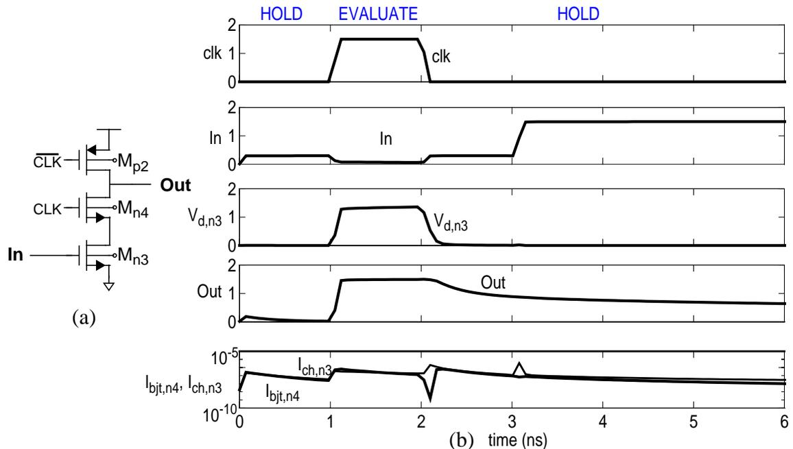
Figure 4-31 Transient bipolar effects of  $[\text{DP}]^2$  logic. (a) Schematic of  $[\text{DP}]^2$  inverter and (b) corresponding node voltages and currents.
