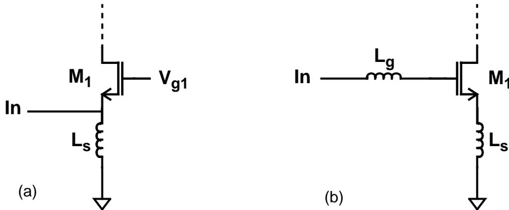
Figure 2-1 Potential CMOS LNA topologies: (a) common-gate or (b) common-source with inductive degeneration.
