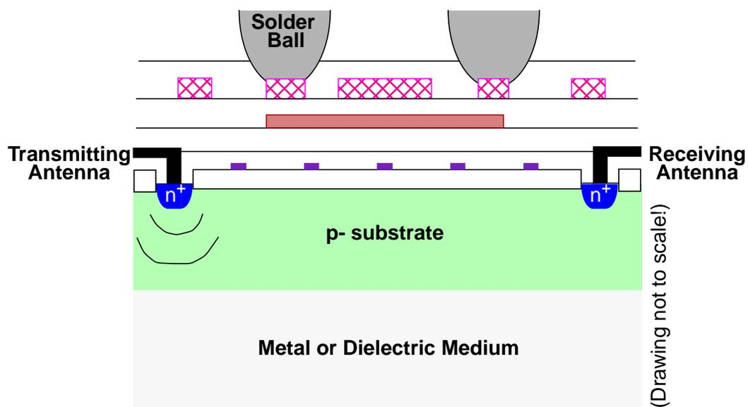
Figure 6-12 Cross-sectional illustration of antennas in direct contact with substrate.
