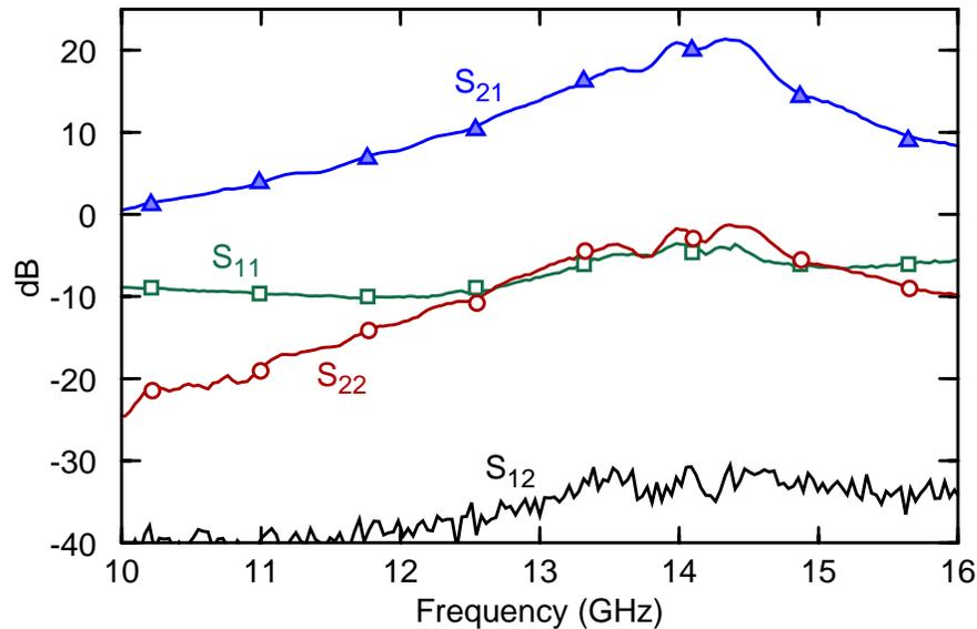
Figure 3-17 Measured S-parameters for differential LNA with source-follower buffers.
