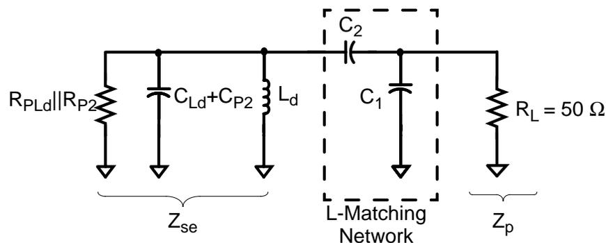
Figure B-2 Small-signal model of common-gate low noise amplifier.
