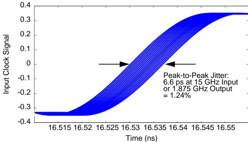
Figure 6-31 Illustration of the measured jitter of the wireless clock receiver. This jitter was measured off of the 15-GHz input signal, yielding the jitter of the 1.875-GHz output signal used as the trigger. The measured peak-to-peak jitter was 6.6 ps.
