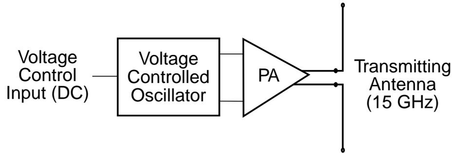
Figure 6-17 Block diagram of clock transmitter for 0.18- $\mu\text{m}$  test chip.
