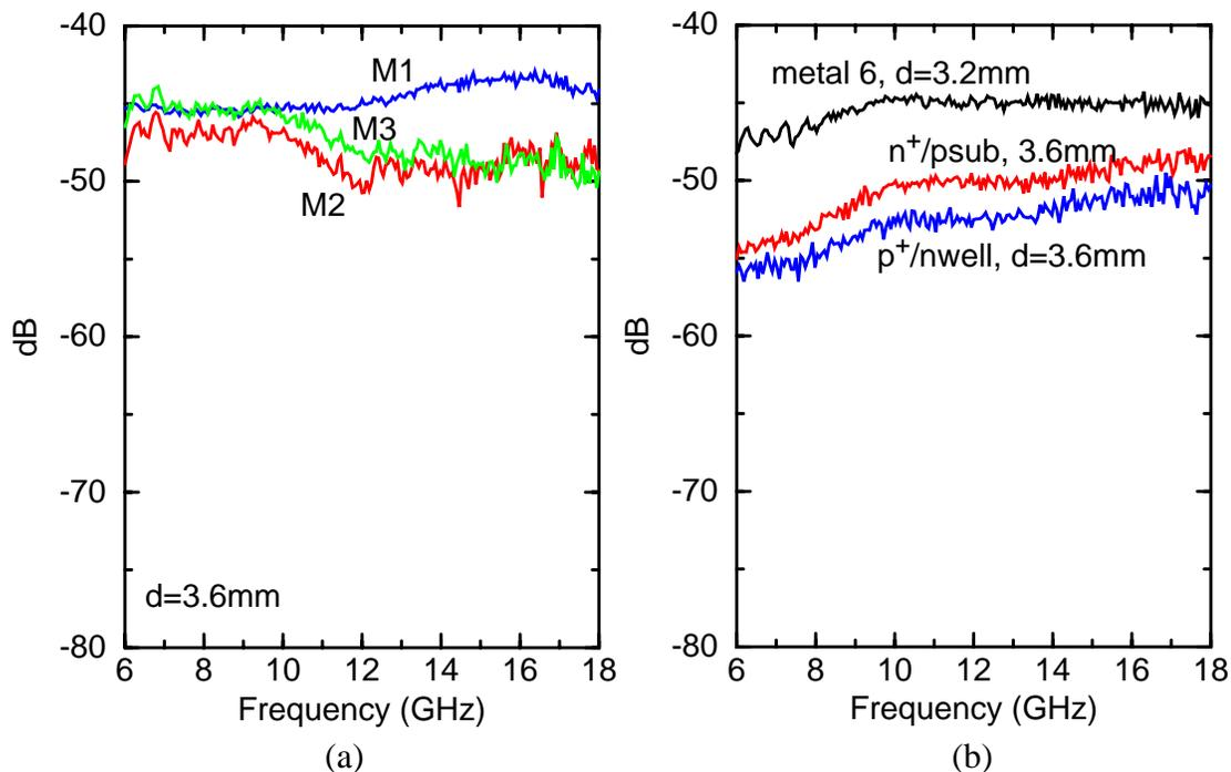
Figure 6-16 (a) Zigzag transmission gains at  $d=3.6$  mm for antennas in metals 1, 2, or 3. (b) Zigzag transmission gains at  $d=3.65$  mm ( $Z_{pp}$ ,  $Z_{np}$ ) for antennas implemented in direct contact with substrate, with n-plus in p-sub and p-plus in n-well. Metal-6 antenna at  $d=3.2$  mm is shown for comparison purposes.
