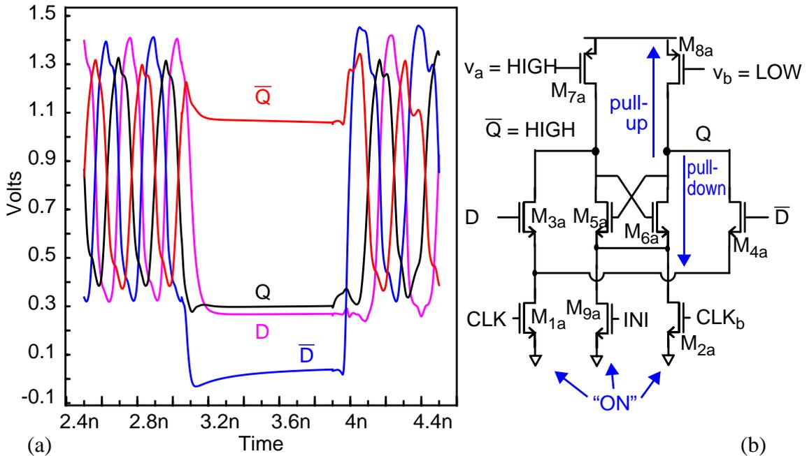
Figure 4-23 (a) Simulated waveforms of programmable 2:1 divider during state-dependent initialization failure. (b) Schematic of DFF indicating conflict of states.
