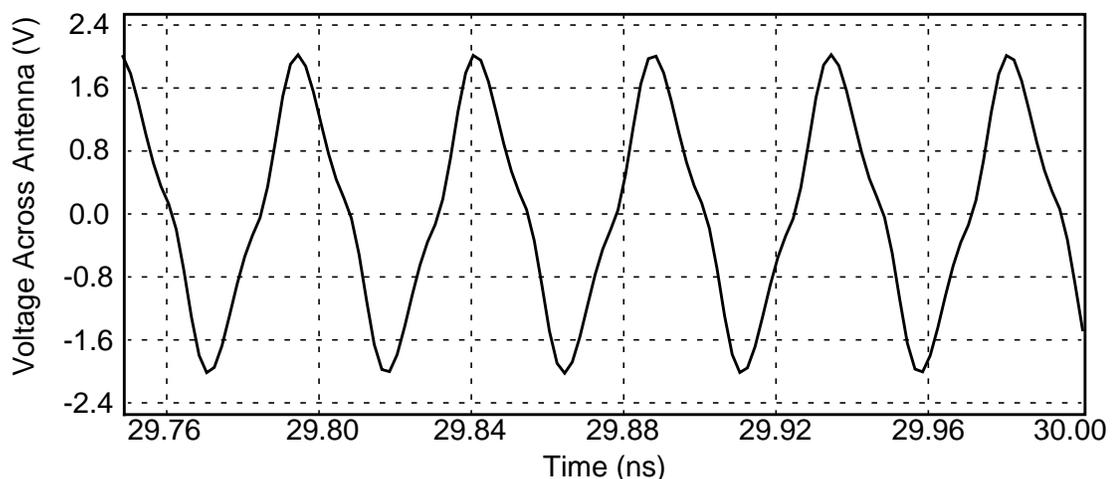
Figure 6-22 A simulated output waveform across the antenna from the PA.
