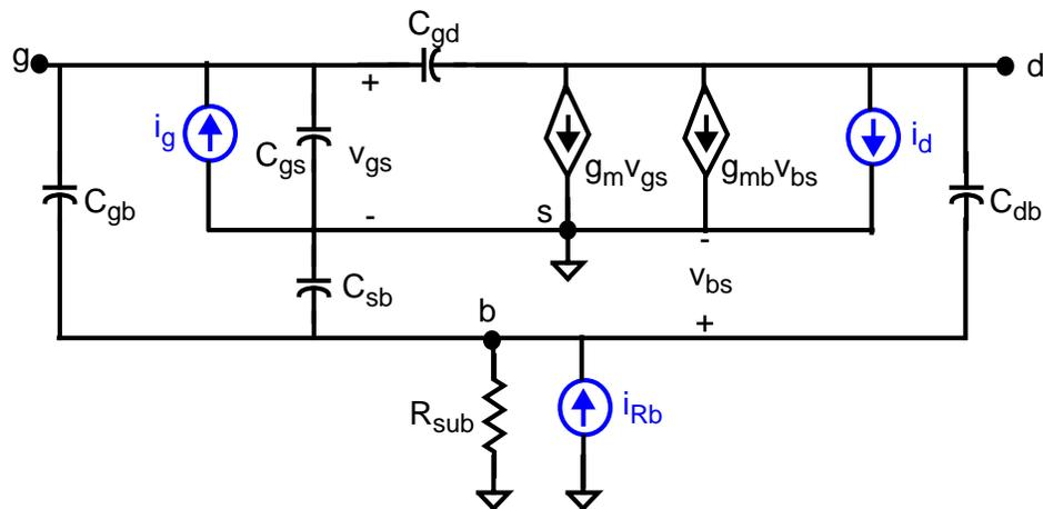
Figure 2-6 High-frequency, quasi-static model of intrinsic MOSFET.
