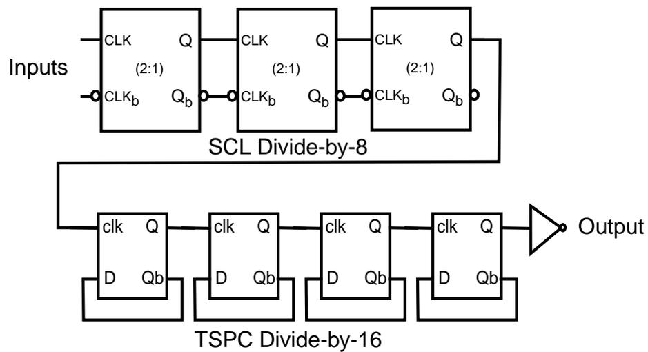
Figure 4-5 Block diagram of 128:1 divider.
