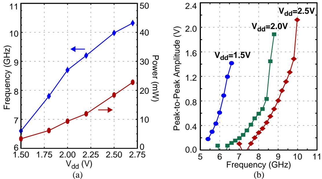
Figure 4-9 Measured results for 0.25- $\mu\text{m}$  divider: (a) Maximum input frequency and power consumption versus supply voltage. (b) Input sensitivity versus frequency versus supply voltage.
