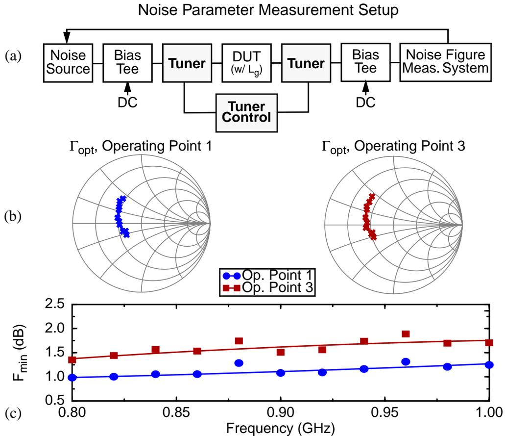
Figure 3-6 (a) Measurement system used to obtain  $F_{min}$  and  $\Gamma_{opt}$ .
