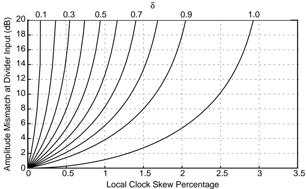
Figure 5-5 Amplitude mismatch allowed at divider input versus local clock skew percentage, with  $\delta$  varying from 0.1 to 1 in 0.1 increments.
