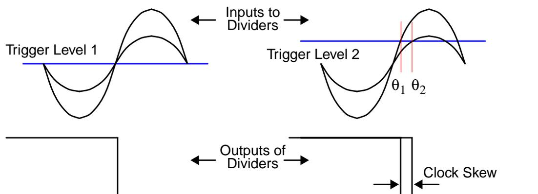
Figure 5-4 Illustrations of AM-to-PM conversion for a divider operating in the latched mode with trigger levels either at the zero crossing (left) or not (right).
