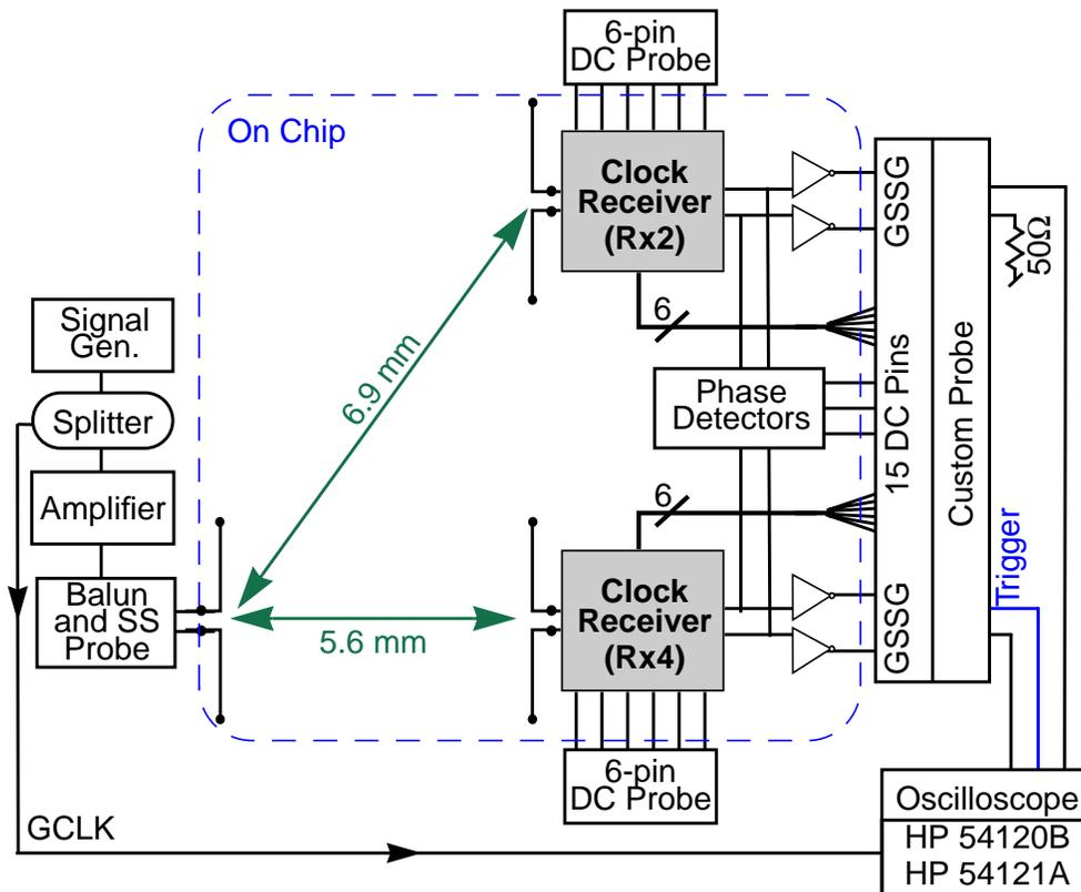
Figure 6-27 Diagram of measurement setup developed for double-receiver interconnect.
