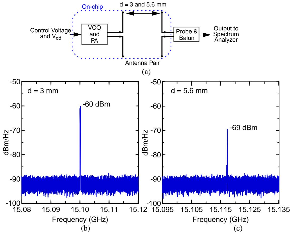
Figure 6-24 (a) Measurement setup used to characterize wireless clock transmitter. (b) & (c) Output spectra from receiving antenna detected from clock transmitter across a 3- & 5.6-mm distance.
