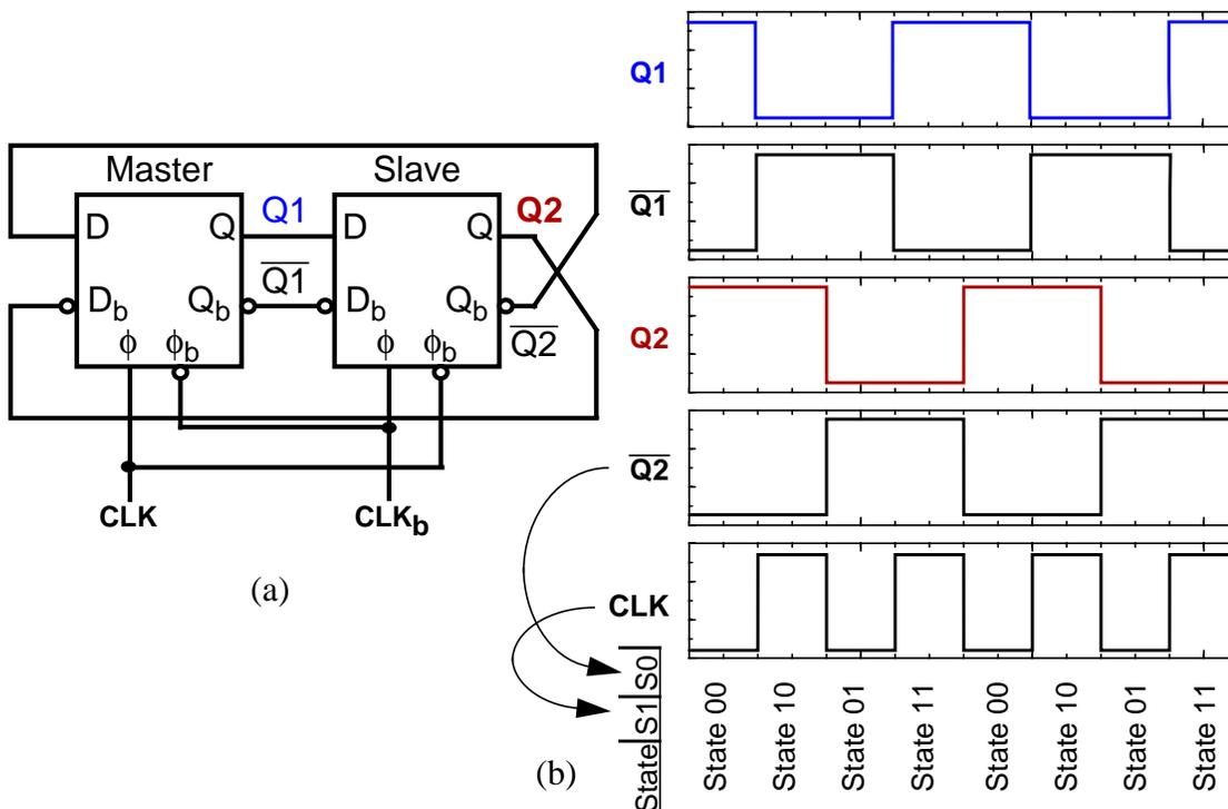
Figure 4-17 (a) Block diagram of 2:1 frequency divider using SCL and (b) ideal input and output waveforms for divider and associated states.
