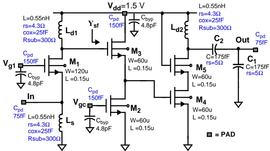
Figure 3-18 Schematic of 23.8-GHz amplifier in a 0.1- $\mu\text{m}$  SOI CMOS technology.
