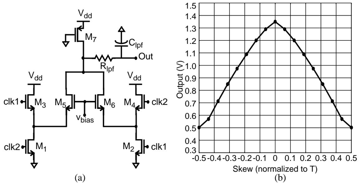
Figure 4-26 (a) Schematic of phase detector and low-pass filter (b) Output of phase detector versus input skew
