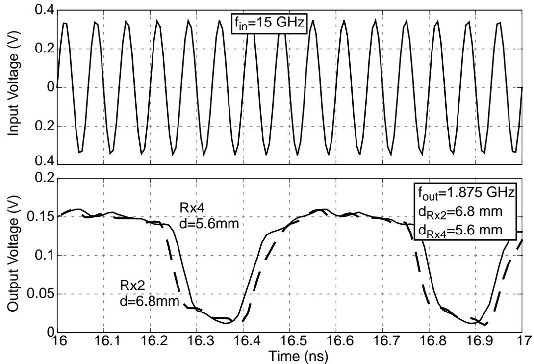
Figure 6-29 Measured input and output waveforms of double-receiver interconnect using  $Z_{6c}$  as the transmitting antenna, with a AlNi as the back dielectric. Input frequency is 15 GHz; output frequencies are 1.875 GHz; distances are 6.8 mm for Rx4 and 5.6 mm for Rx2. Time-of-flight delay mismatch and amplitude mismatch are present.
