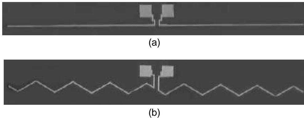
Figure 6-1 Die photograph of (a) linear and (b) zigzag dipole antennas.
