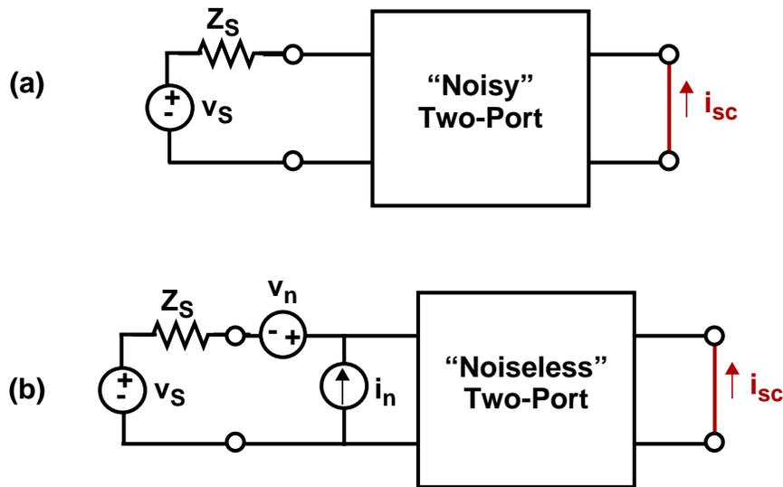
Figure C-1 Representation of a “noisy” two-port network as a “noiseless” two-port with equivalent input noise generators.
