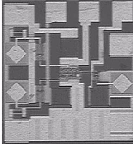
Figure 4-30 Die photograph of 4:1 frequency divider.
