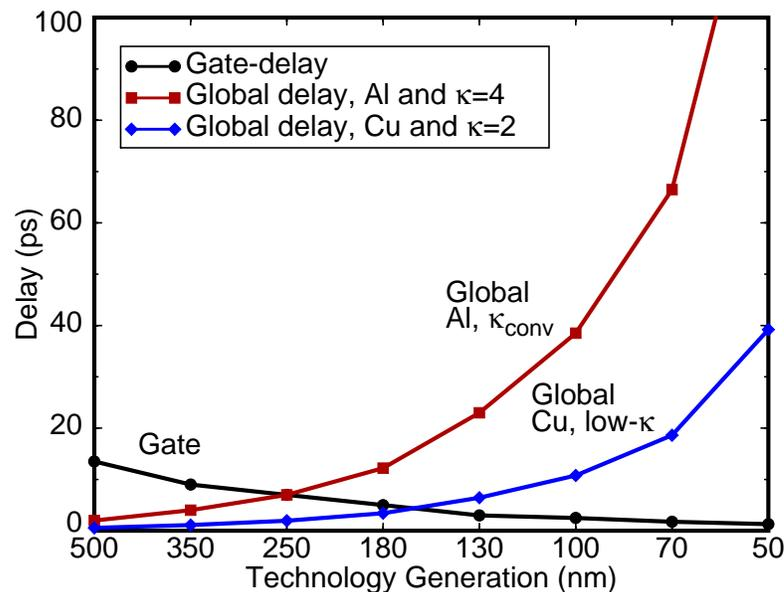
Figure 1-1 Global interconnect delay and gate-delay versus technology generation for aluminum and copper metallization and conventional and low- $\kappa$  dielectrics.
