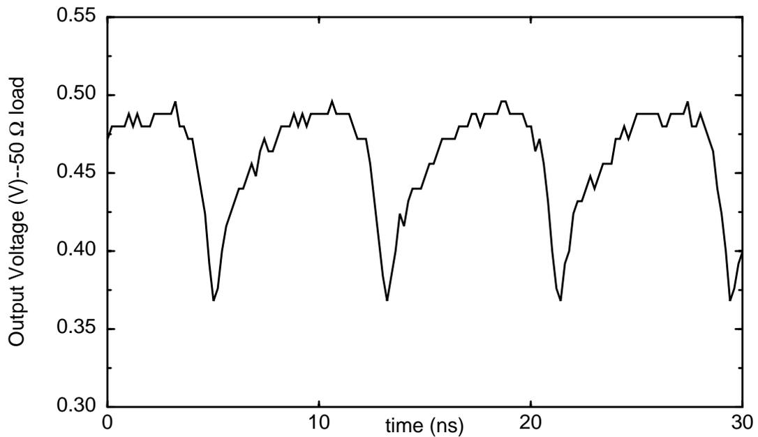
Figure 4-33 Output wave-form for bulk 128:1 frequency divider for 15.36-GHz input signal and  $V_{dd}=1.5$  V. Output frequency is 120 MHz.
