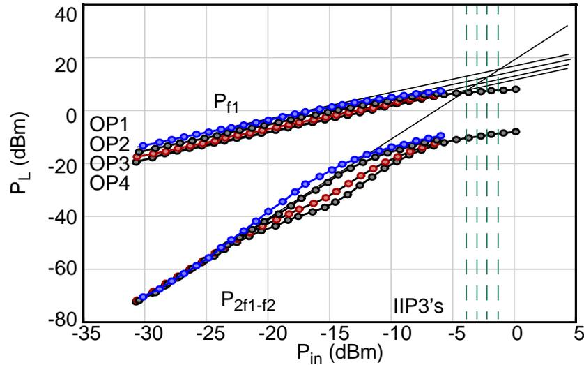
Figure 3-7 Measured  $P_{1dB}$  and IIP3, operating points 1-4.
