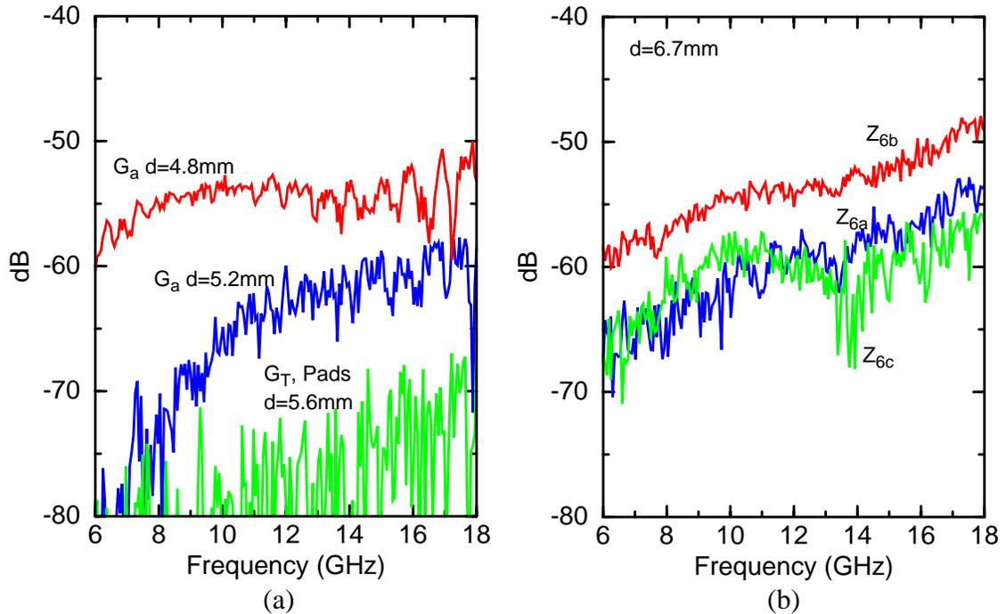
Figure 6-14 (a) Loop-zigzag transmission gains for  $d=5.2$  ( $LP_1$ - $Z_{6f}$ ) and  $4.8$  mm ( $LP_1$ - $Z_{6a}$ ). Also shown is the pad transducer gain ( $|S_{21}|^2$ ) at  $d=5.6$  mm for reference. (b) Zigzag transmission gains for metal-6 antennas ( $Z_{6a,6b,6c}$ ) at  $d=6.7$  mm, demonstrating the effect of interference structures on gain.
