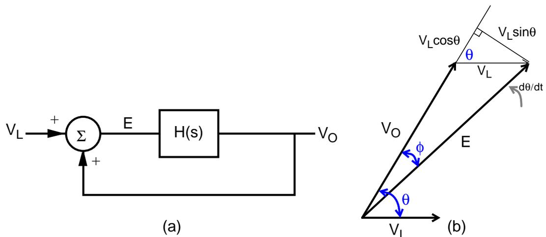
Figure E-1 (a) Basic feedback model of an injection-locked oscillator.
