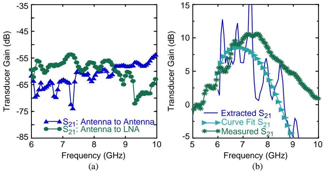
Figure 6-7 (a) Measured transducer gain between antenna pair and antenna pair with LNA. (b) Extracted and measured gain of LNA.
