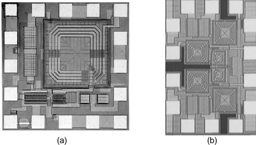
Figure 3-3 Die photographs of (a) 0.8- $\mu\text{m}$ , 900-MHz single-ended CMOS LNA and (b) 0.25- $\mu\text{m}$ , 8-GHz differential CMOS LNA.
