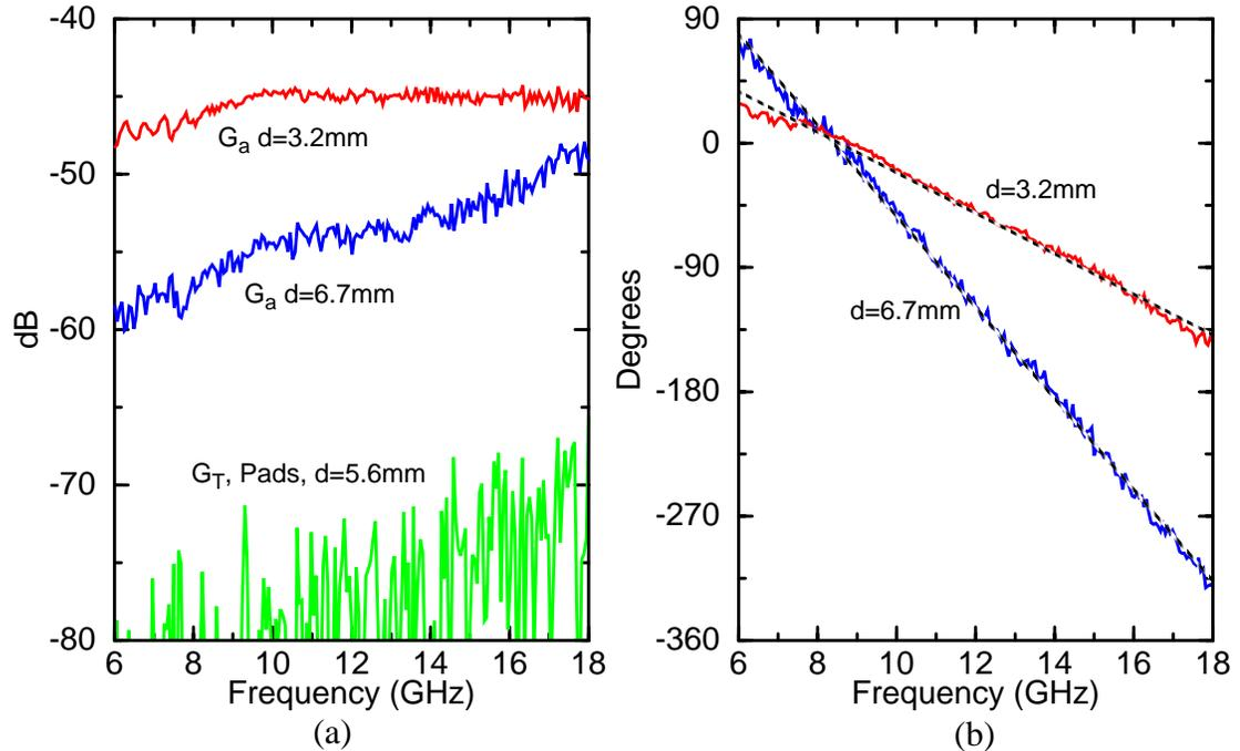
Figure 6-13 (a) Zigzag-zigzag transmission gains for  $d=6.7$  mm ( $Z_{6b}$ ) and 3.2 mm ( $Z_{6c-6f}$ ). Also shown is the pad transducer gain ( $|S_{21}|^2$ ) at  $d=5.6$  mm for reference. (b) Phase versus frequency of voltage wave for  $d=6.7$  and 3.2 mm.
