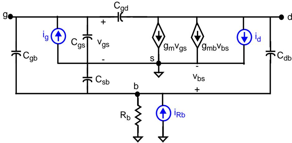
Figure D-1 High-frequency, quasi-static model of intrinsic MOSFET [Tsi99].
