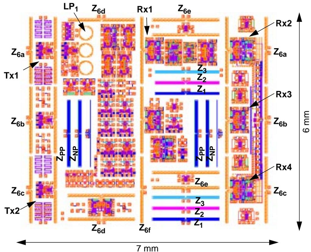
Figure 6-10 Layout of UMC test-chip showing locations of relevant zigzag antennas ( $Z_x$ ), loop antenna ( $LP_1$ ), clock transmitters (Tx), and clock receivers (Rx).
