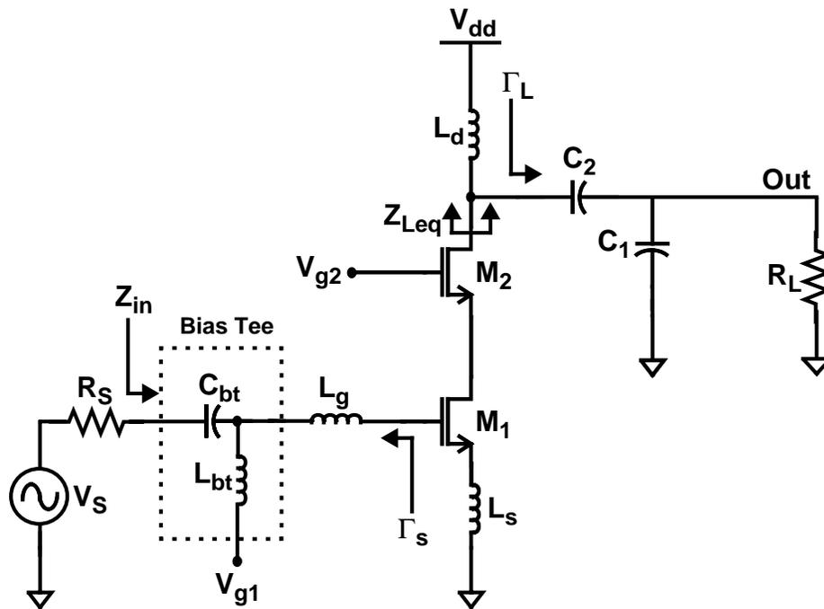
Figure 2-2 Schematic of the source-degenerated CMOS LNA
