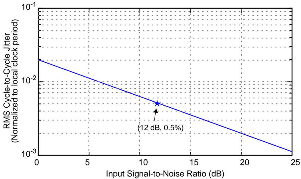
Figure 5-7 Local clock jitter versus signal-to-noise ratio at input to divider.
