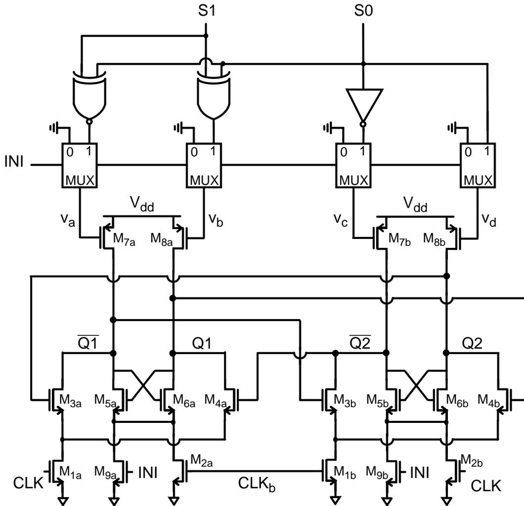
Figure 4-18 Schematic of 2:1 frequency divider with initialization circuitry.
