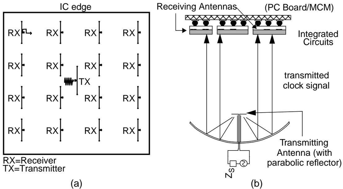
Figure 1-2 Conceptual system illustrations of (a) intra-chip and (b) inter-chip wireless interconnect systems for clock signal distribution.
