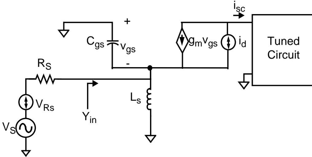
Figure A-1 Small-signal model of common-gate low noise amplifier.
