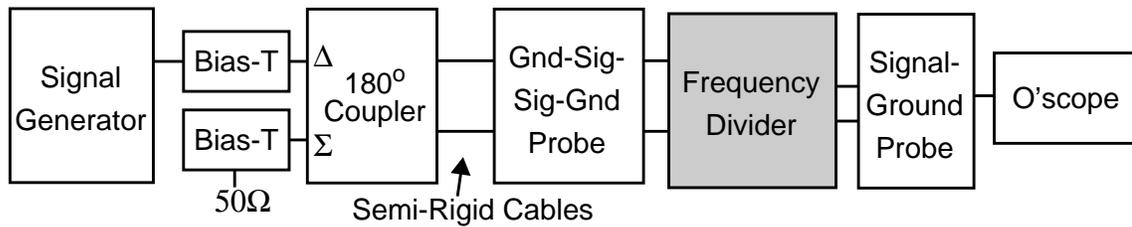
Figure 4-8 Measurement setup used to characterize dual-phase frequency divider.
