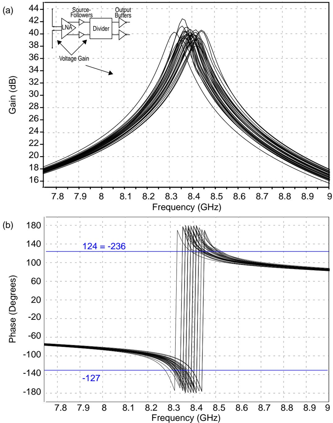
Figure 7-6 Simulated process variation of (a) voltage gain and (b) phase-shift of receiver from antenna input to input of frequency divider.
