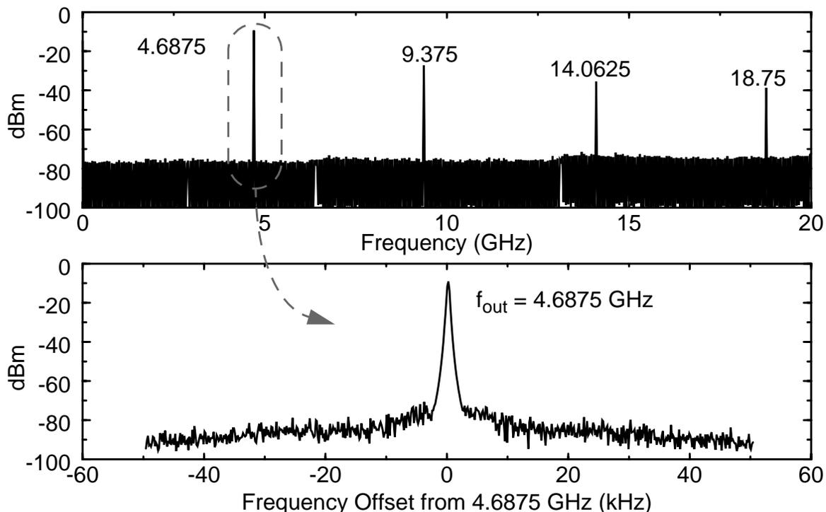
Figure 4-32 Output spectrum of SOI 4:1 frequency divider for  $f_{in} = 18.75$ -GHz and  $V_{dd} = 1.5$  V.
