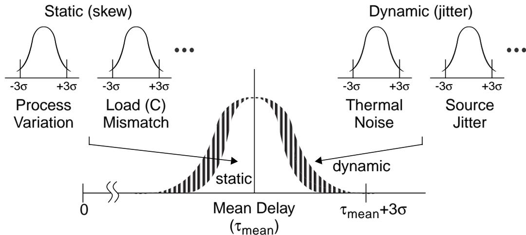
Figure 5-3 Probability density function of propagation delay, including both static and dynamic components resulting in clock skew and jitter (after EDN, July 1995, pp. 35).
