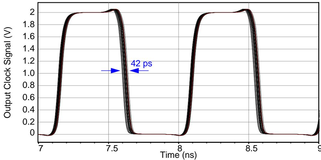
Figure 7-5 Process variation of frequency divider, obtained with Monte Carlo analysis (30 iterations), for an 8.5-GHz, 500-mV amplitude input signal,  $V_{dd} = 2$  V.
