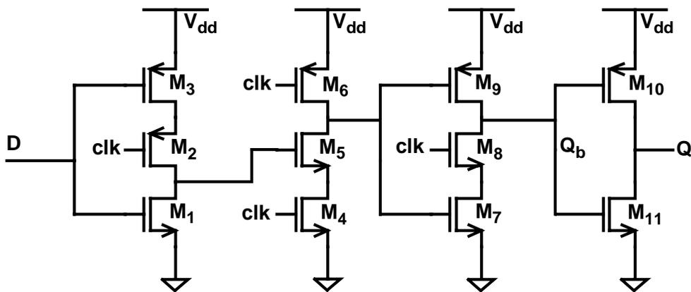
Figure 4-6 Schematic of true single-phase clocked (TSPC) latch.
