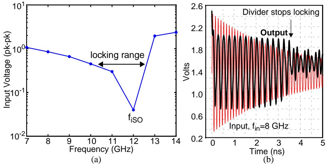
Figure 4-4 (a) Simulated input sensitivity of 0.25- $\mu\text{m}$  CMOS 8:1 divider (b) Exponentially decreasing input signal at 8 GHz and output signal of 8:1 divider, illustrating divider's dependence on input voltage swing.
