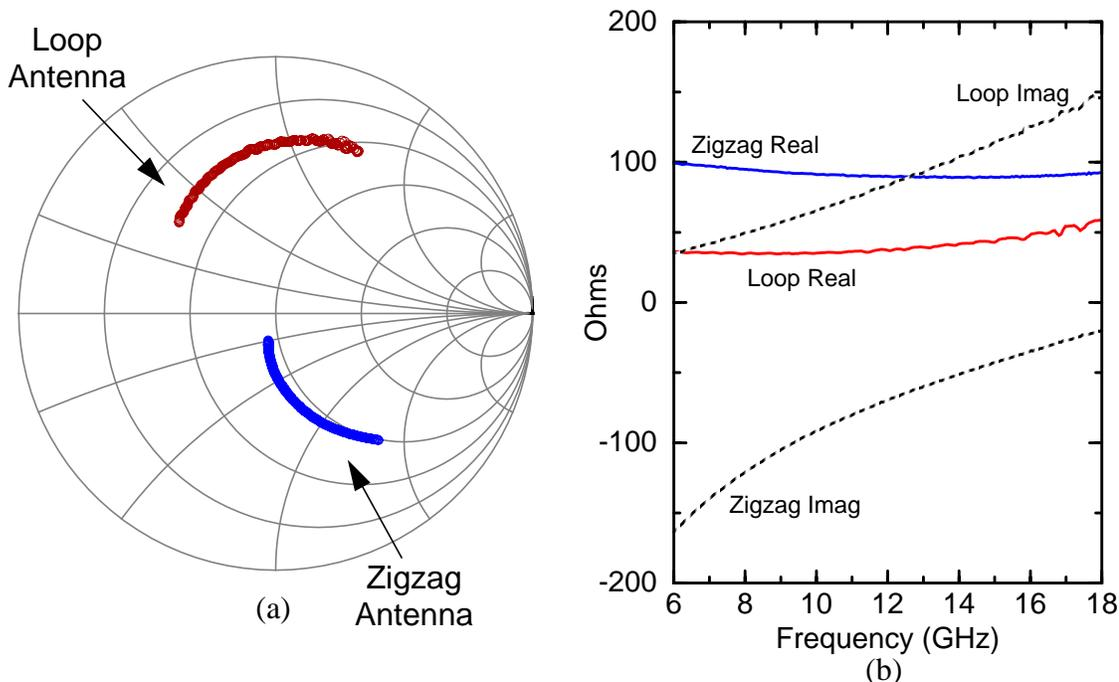
Figure 6-15 (a) Impedance smith chart showing reflection coefficients of zigzag and loop antennas (Impedances are normalized to 100  $\Omega$ ). (b) Antenna impedance for zigzag and loop antennas ( $Z_{6b}$  and  $LP_1$ ).
