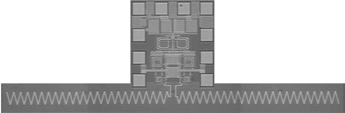
Figure 6-18 Die photograph of 0.18- $\mu\text{m}$  clock transmitter with zigzag dipole antenna.
