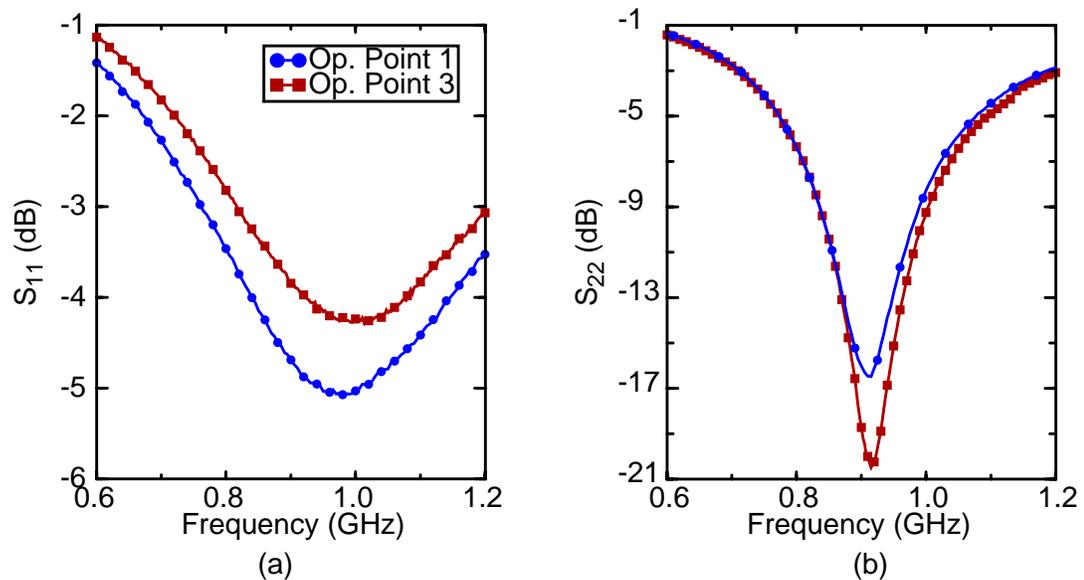
Figure 3-5 (a) Input ( $S_{11}$ ) and (b) Output ( $S_{22}$ ) reflection coefficients versus frequency, operating points 1 and 3.
