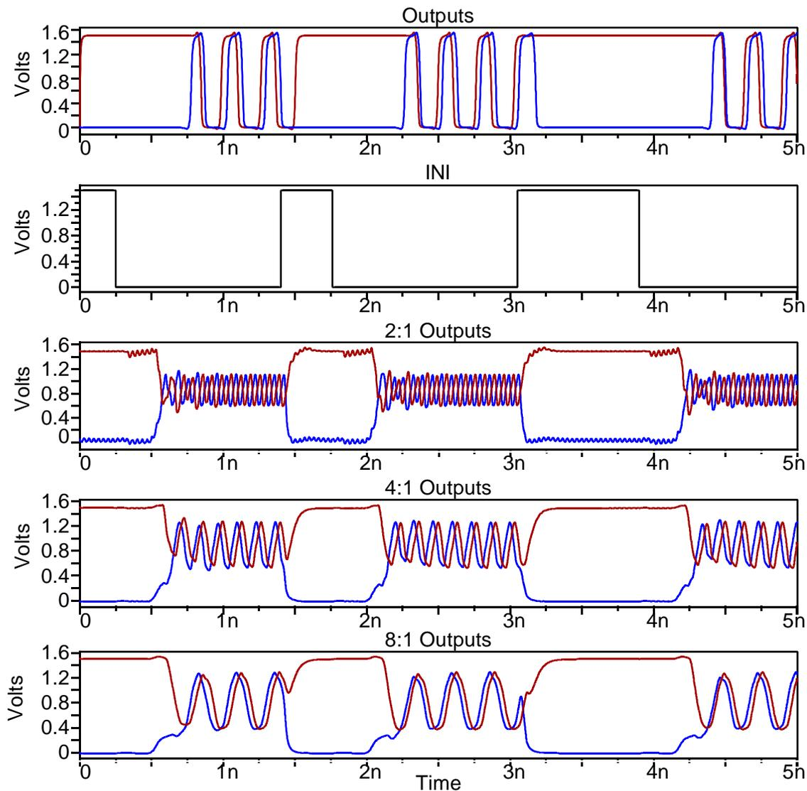
Figure 4-25 Simulated waveforms of two programmable 8:1 dividers with the new DFFs--programmed to #000 (solid lines) and #111 (dashed lines)--for repeated initializations. The circuit functions correctly and the output phase difference between the two dividers remains constant.
