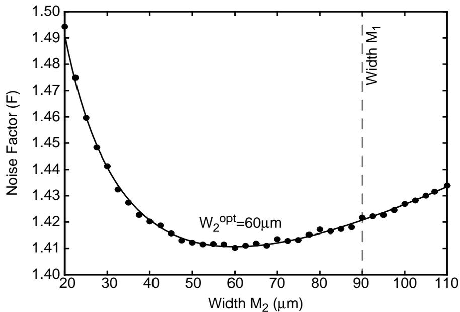
Figure 2-9 Noise factor versus width of cascoded transistor ( $M_2$ ). The optimum width occurs when the capacitance at the intermediate node between  $M_1$  and  $M_2$  is equally balanced between  $M_1$  and  $M_2$ .
