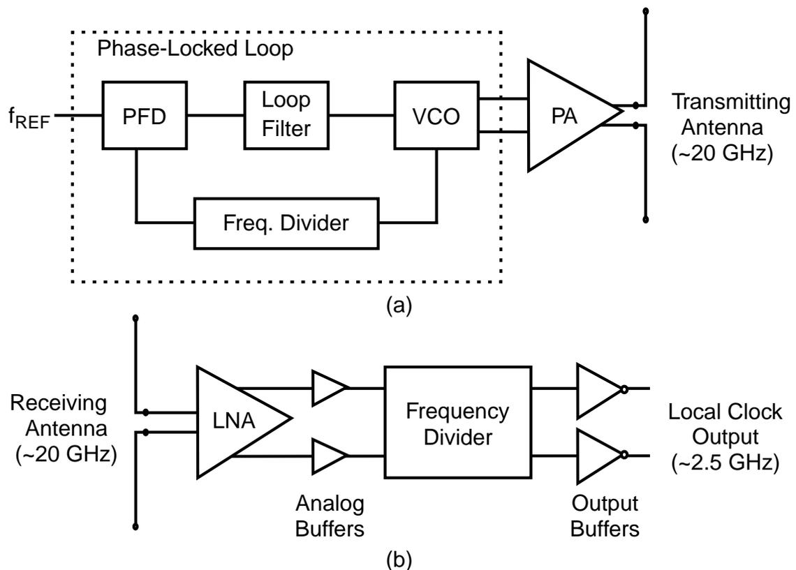
Figure 1-3 Block diagrams of (a) integrated clock transmitter and (b) integrated clock receiver.
