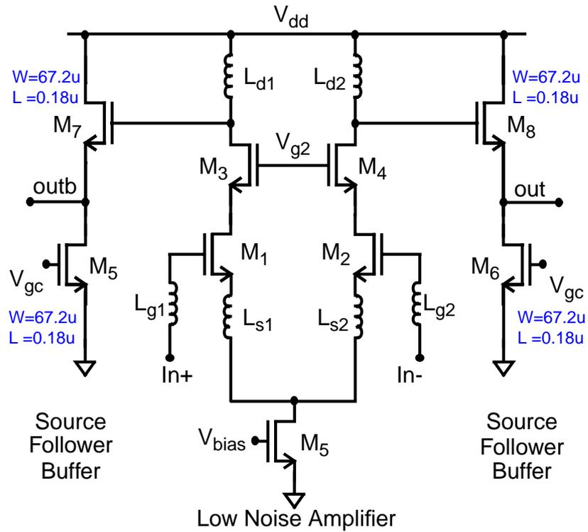
Figure 3-12 Schematic of differential 14-GHz LNA with source-followers.
