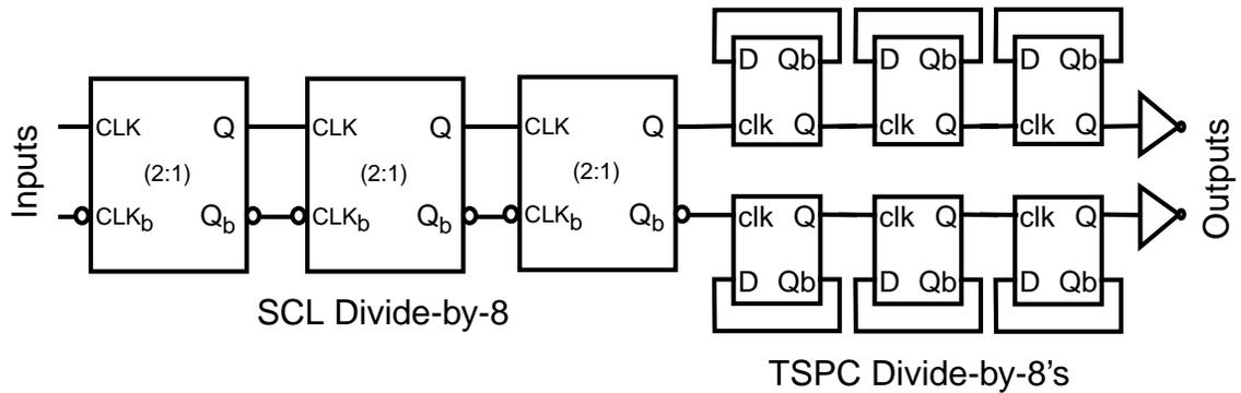
Figure 4-11 Block diagram of 64:1 divider implemented in 0.18- $\mu\text{m}$  CMOS technology.
