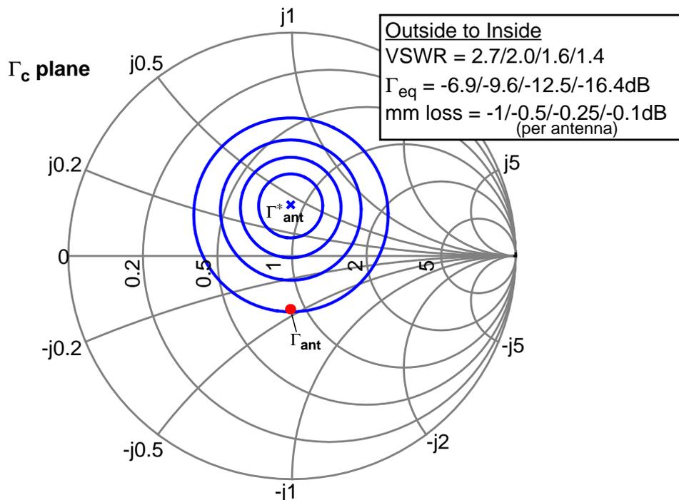
Figure 5-2 Constant  $\Gamma_{eq}$  circles in the  $\Gamma_c$  plane. This shows the allowable circuit impedances for a given antenna reflection coefficient ( $\Gamma_{ant}$  for  $z_{ant}=(89-j45)/100$ ).
