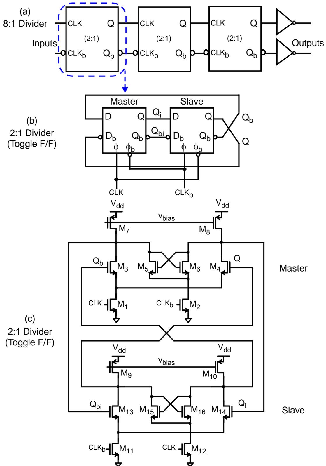
Figure 4-1 Block diagrams of (a) 8:1 divider consisting of three cascaded 2:1 dividers, and (b) 2:1 divider consisting of two D-latches in master/slave. (c) Schematic of 2:1 divider implemented using source-coupled logic.
