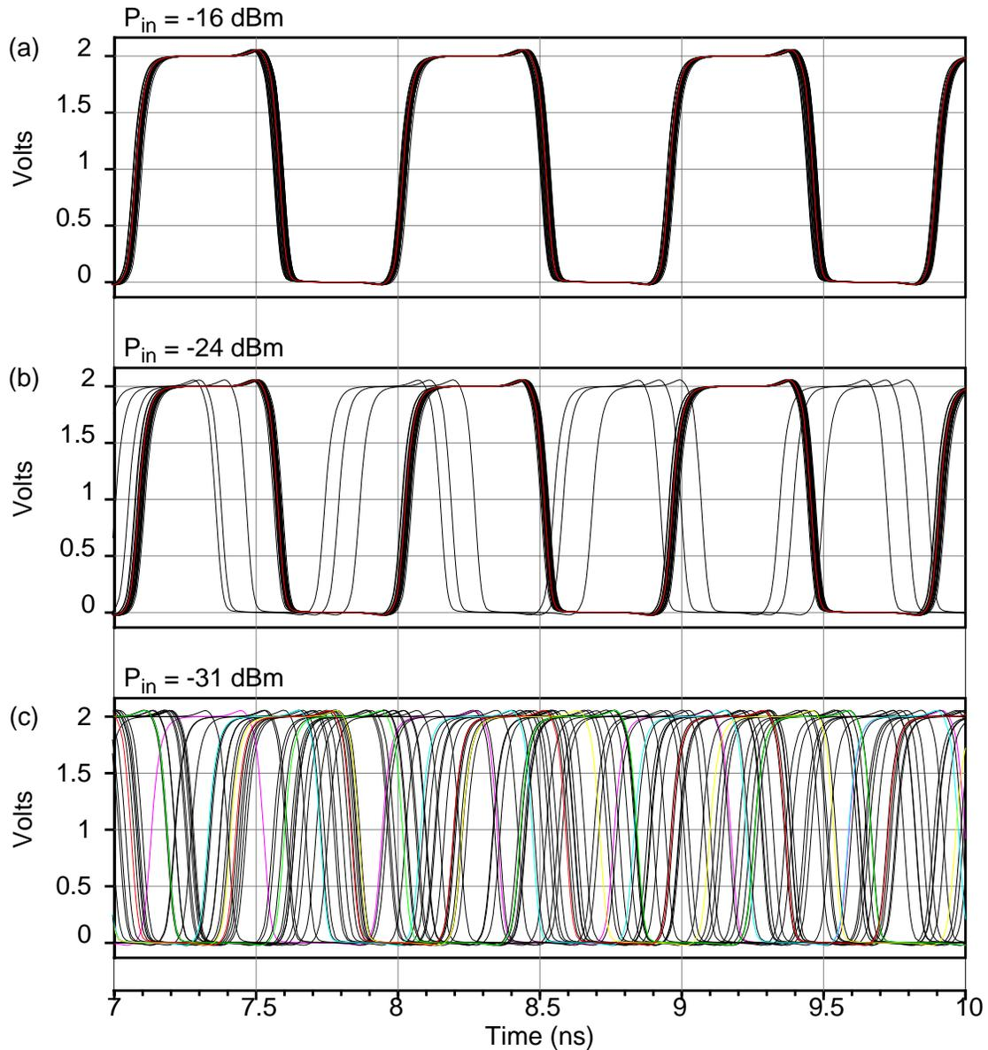
Figure 7-7 Output clock signals from frequency divider with process variation: Input power levels are (a) -16 dBm, (b) -24 dBm, (c) -31 dBm.
