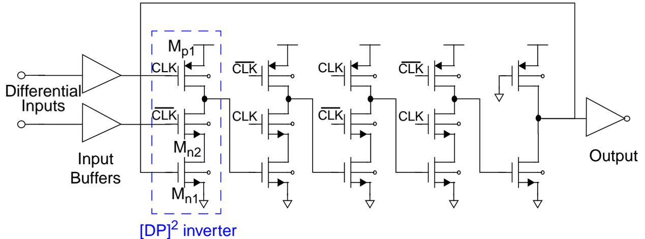
Figure 4-29 Schematic of 4:1  $[DP]^2$  synchronous divider.
