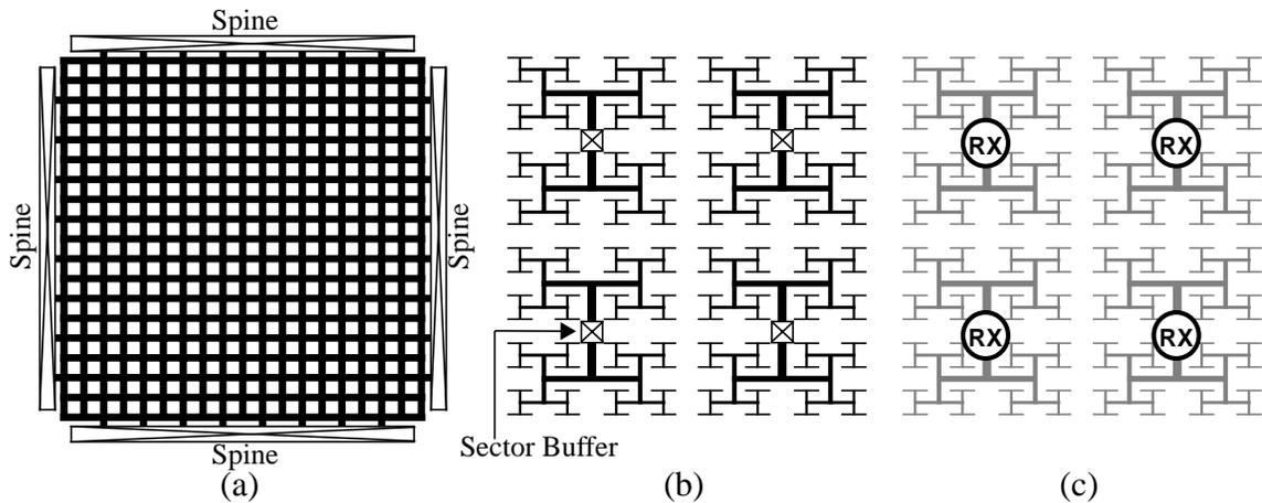
Figure 7-3 Illustration of *single quadrant* of global clock distribution systems for (a) grid, (b) H-tree, and (c) wireless.
