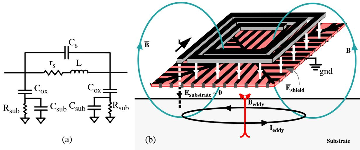
Figure 3-1 (a) General two-port lumped-element model for spiral inductor. (b) Illustration of a spiral inductor above a patterned-ground shield. The shield terminates most of  $\vec{E}$ -field while allowing  $\vec{B}$ -field to pass through, increasing  $Q$ .
