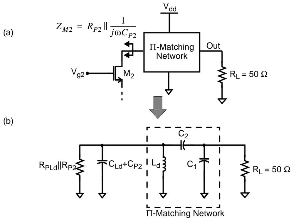
Figure 2-4 Output matching equivalent circuits for CMOS LNA
