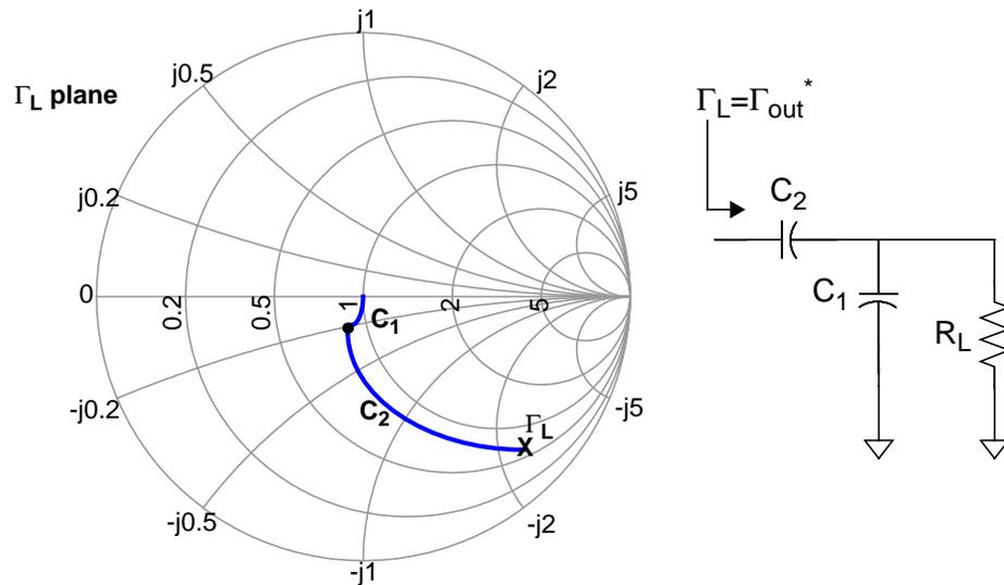
Figure 2-12 Output matching network design to match  $50\ \Omega$  to  $\Gamma_{out}^*$ .
