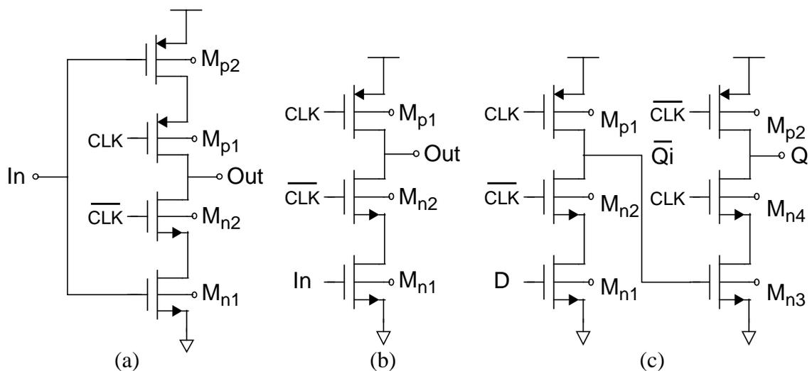
Figure 4-28 Schematics of (a) C<sup>2</sup>MOS inverter, (b)  $[DP]^2$  inverter or level-sensitive latch and (c)  $[DP]^2$  edge-triggered D-Flip-Flop
