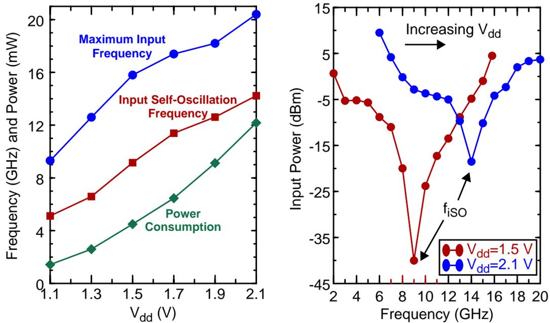
Figure 4-13 Measured results of 0.18- $\mu$ m frequency divider
