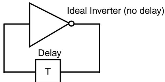
Figure F-1 Model of ring oscillator as an ideal inverter followed by a delay element, used to find the Q of a ring oscillator.
