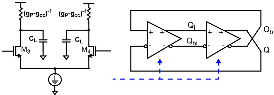
Figure 4-2 Representation of source-coupled latch as a fully-differential amplifier and the 2:1 divider as an oscillator.
