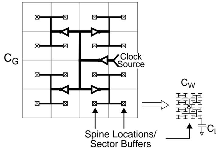
Figure 7-1 Illustration of total global clock capacitance.
