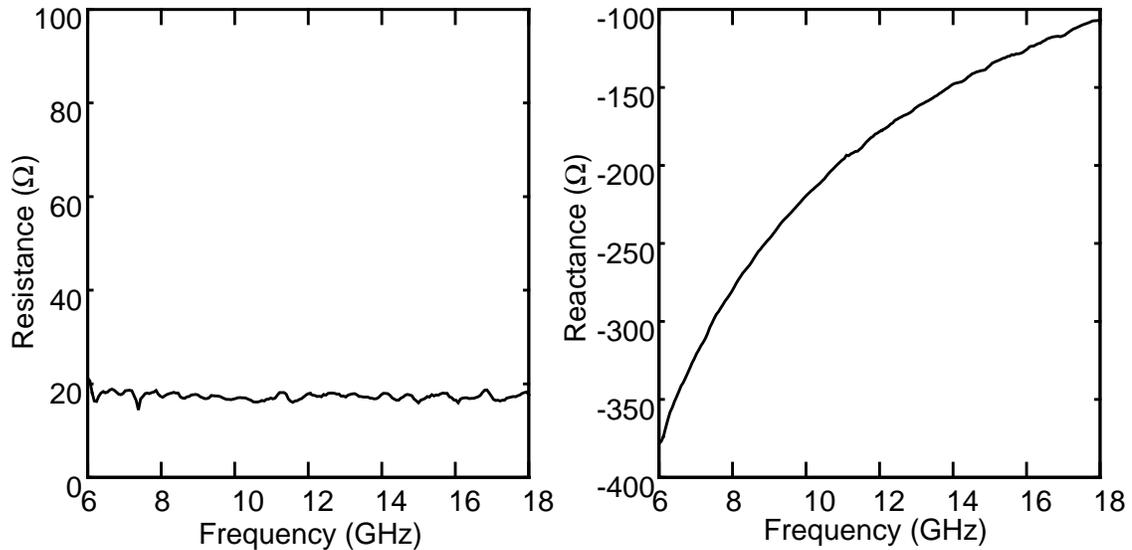
Figure 6-6 Antenna impedance versus frequency for linear dipole antenna.
