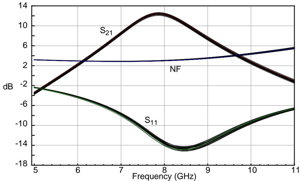
Figure 7-4 Process variation of single-ended LNA's gain ( $S_{21}$ ), noise figure (NF), and input matching ( $S_{11}$ ), obtained with Monte Carlo analysis (30 iterations).
