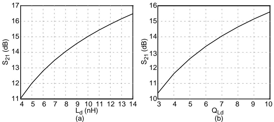
Figure 2-5  $S_{21}$  at resonance versus (a)  $L_d$  for constant  $Q_{Ld}$  and (b)  $Q_{Ld}$  for constant  $L_d$ . The output is always matched to  $50 \Omega$ .
