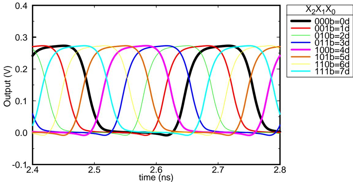
Figure 4-21 Output waveforms of 8:1 divider for each start-up condition
